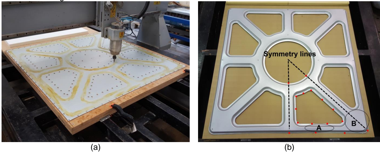
Fig.2: (a) Incremental forming of the 0.4 mm sheet using a CNC router and (b) the final incrementally formed support showing the points where distortions were measured.
