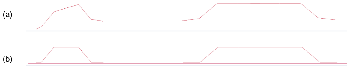
Fig.15: A cross-section at A-A in Figure 6 of the (a) distorted geometry used in simulations #3 to #5 and (b) the undistorted geometry used in simulation #1.
