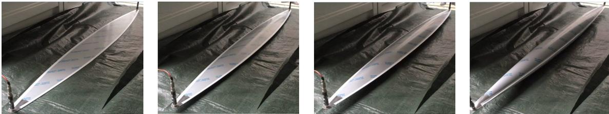
Fig.5: Sequence of the forming experiment with specimen 0160 resulting in a completely buckle-free Die-Less-Hydroforming object that can be used as an outer shell for the Hybridcolumn PERFECTO (Source: [2])
