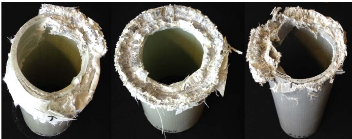
Fig.8: Axial compression of circular pultruded tubes with length 239 mm.
