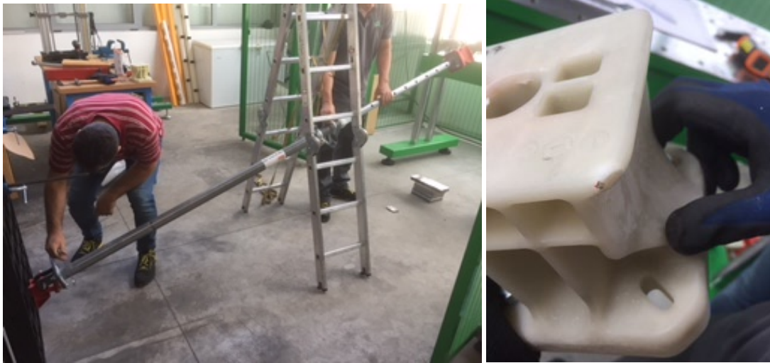
Fig.8: Experimental layout in Polytech Laboratories to reproduce the impact conditions analyzed in simulation (left) and impacted exemplar (right)
