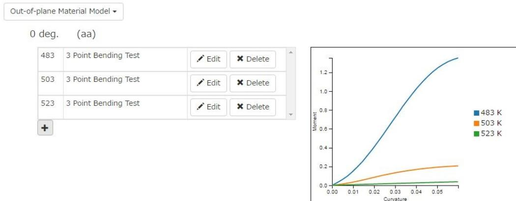
Fig.2: GUI for the input of temperature dependent mechanical properties
