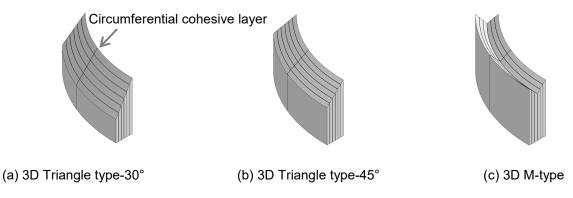
Fig.2: 3D models of triggered FRP tube
