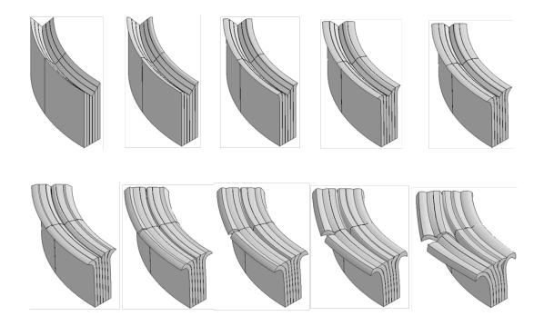
Fig.7: Failure behaviours of 3D M-type model
