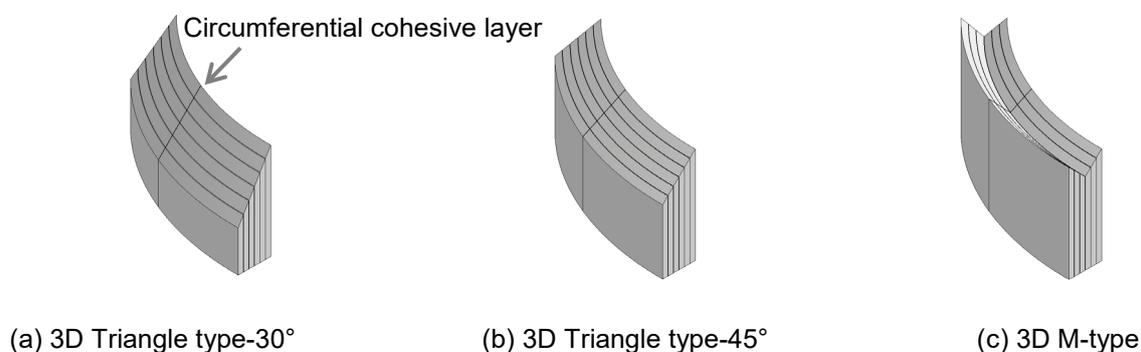
Fig.2: 3D models of triggered FRP tube
