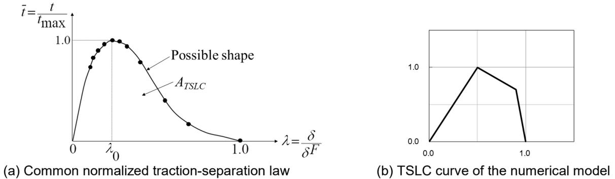
Fig.3: Normalized traction-separation law (TSLC) of MAT\_186
