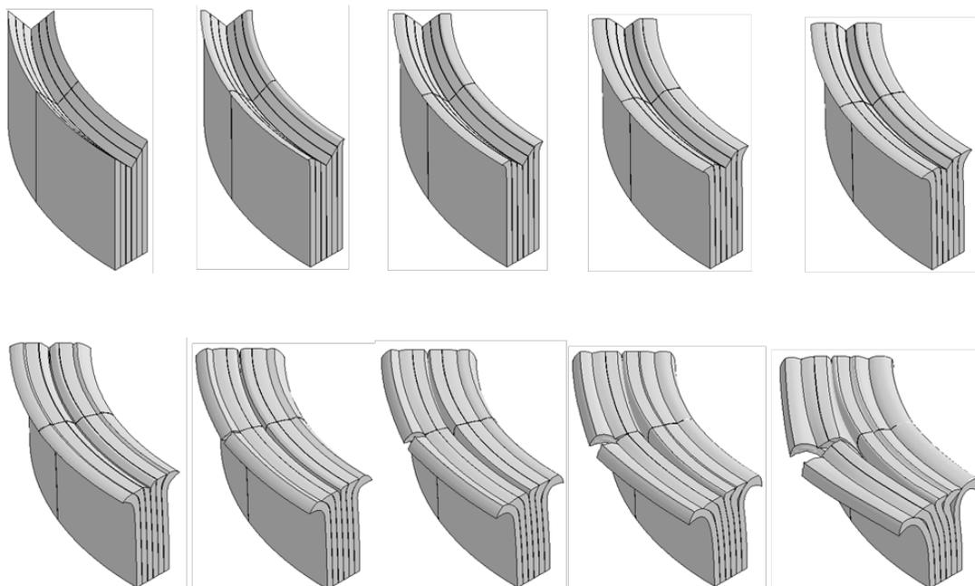
Fig.7: Failure behaviours of 3D M-type model
