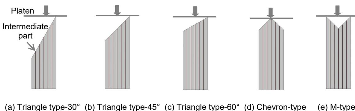
Fig.1: Plate models of triggered FRP tube and loading condition
