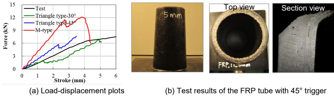
Fig.6: Load-displacement plots by simulation and test results of the FRP tube
