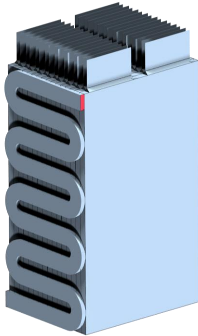
Fig.3: CAD model of the test setup consisting of 16 battery cells and a cooling channel
