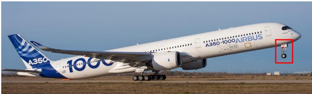
Currently this part is categorized in class 1. This means that the failure of the actuator leads to a failure of the chassis, which is a catastrophic event. Table 1 shows the categorization of components based on the consequence of a failure:
