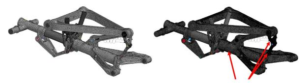
The model with the coarse mesh runs in 7 hours by using 16 cores in parallel. This model is sufficient to calculate the forces acting on the interface to the airplane body.
