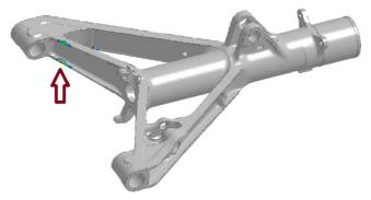
In one point we can see a sensitive behavior of the model: Small differences e.g. in the meshing or modeling of friction lead to a different behavior of the locking strut. In some situation the locking strut locks immediately after the full extension and stays locked until the end. In other situation the locking strut springs up again because of the vibrations in its environment.
