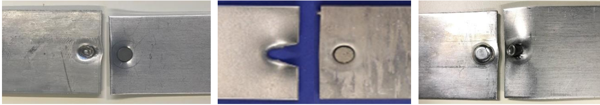
Fig.4: SPR joint failure modes, (from left to right) V1, V2, V3
