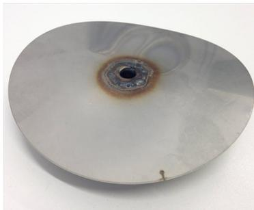
(e) welding distortion for a circular test welding in the center of a circular blank (here:  $d=110$  mm,  $t=0,8$  mm) made of 1.4301 without any fixation
