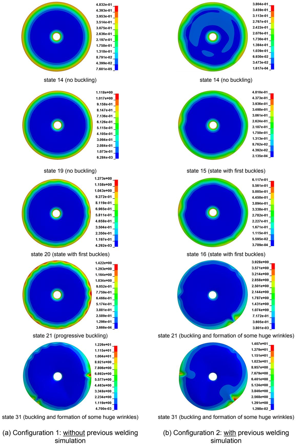
Fig.6: Visualization of the development of buckling at the outer edge of the samples in terms of in-plane-displacement [mm] for different states of inflation
