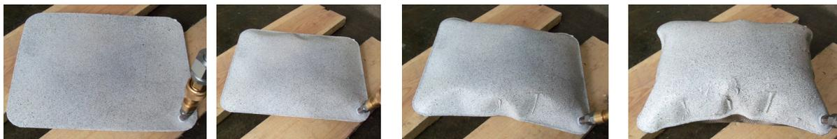
(b) practical test with a double-layered thin stainless steel blank (1.4301) transforming to a pillow-like structure by inflating, here painted with a speckle-pattern for Digital Image Correlation (DIC)-measurement [11]
