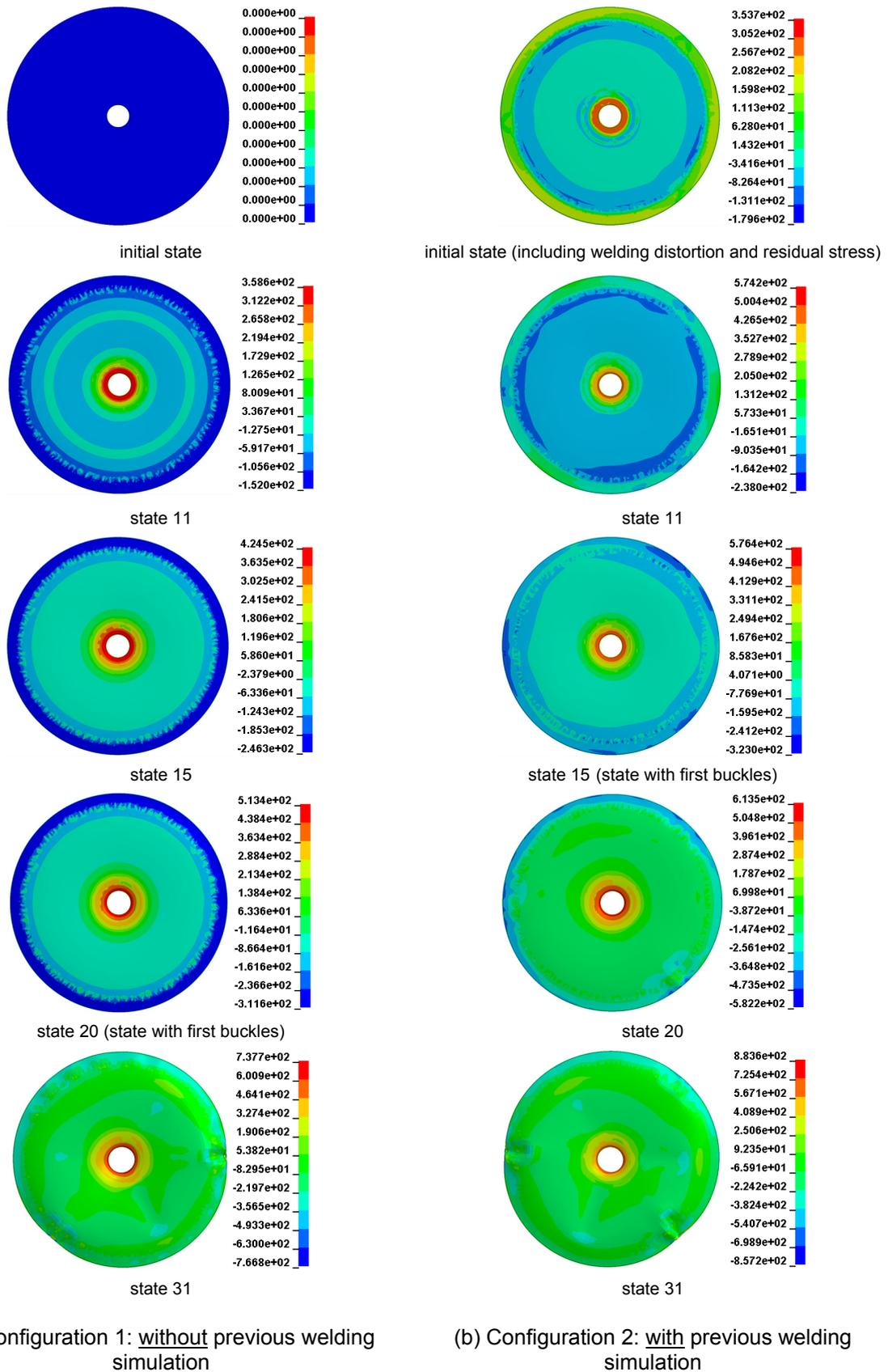
Fig.5: Local element true stress [MPa] in “circumferential direction” of the circular ring sample (midplane integration point) for different states during the inflation
