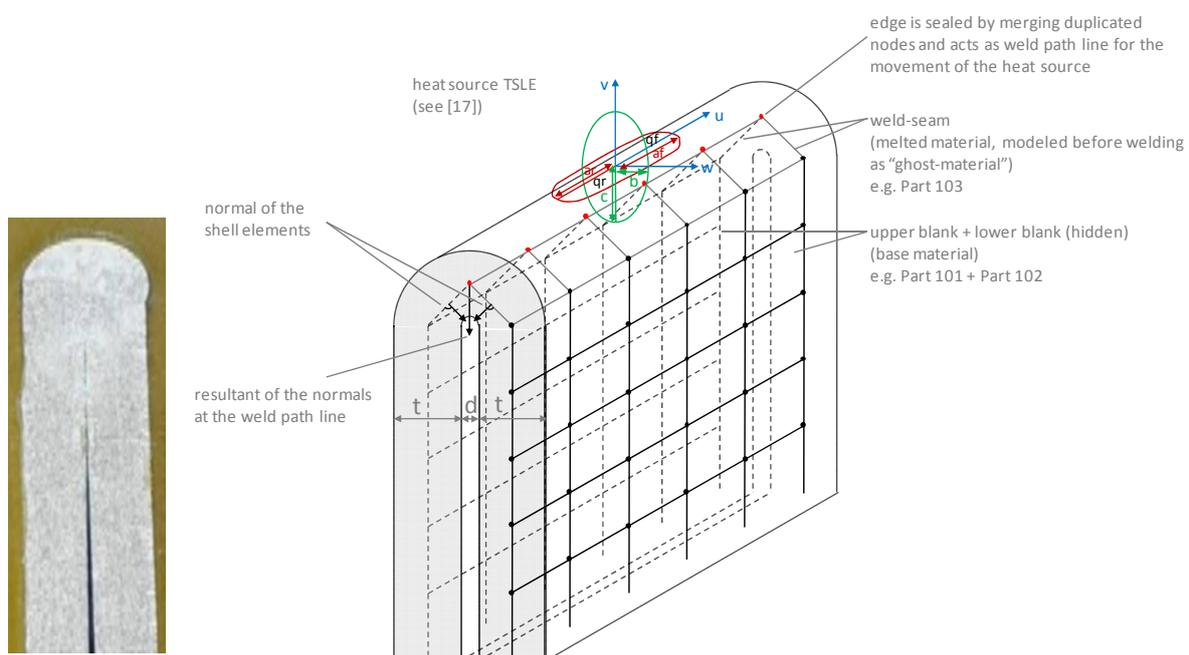
Fig.2: Modeling scheme of a double-layered “Die-Less-Hydroforming” blank (taken from [11] and supplemented) including heat source for welding and a corresponding exemplified macrosection of the face weld, however, additional fixation equipment is not illustrated
