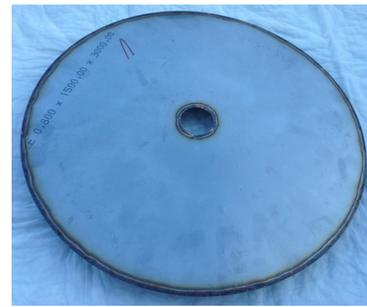
(f) welding distortion of the double-layered "Die-Less-Hydroforming"-blank according to Fig.3: (maximum displacement amplitude normal to surface in the range between approx. 5 up to 6 mm), in this case admittedly welded with fixation by chipboard plates
