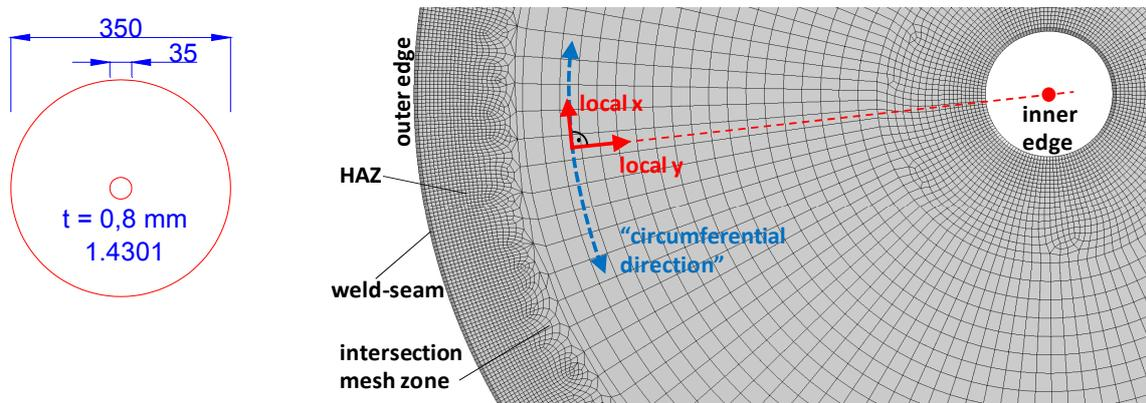
(a) blank geometry [mm] (b) meshing details and orientation of local element coordinate system
