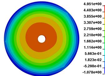
(d) welding distortion [mm] normal to surface after cooling-down to ambient temperature for the model configuration shown in (b)
