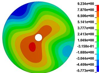
(c) welding distortion [mm] normal to surface after cooling-down to ambient temperature for the model configuration shown in (a)
