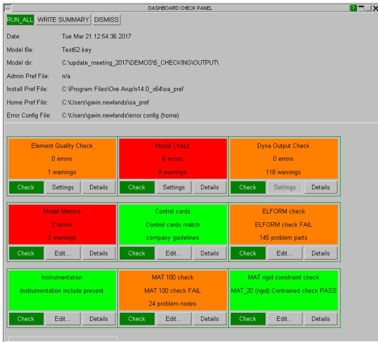
The example shows various checks and whether the model passes the check or not. The scripting based ones are as follows:
