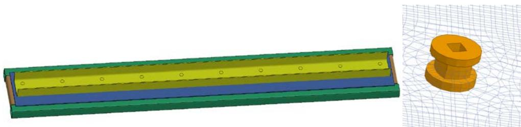
Fig.1: A sandwich structure of dissimilar materials: top aluminum plate in yellow, base steel plate in blue, joined with self-piercing rivets in orange.
