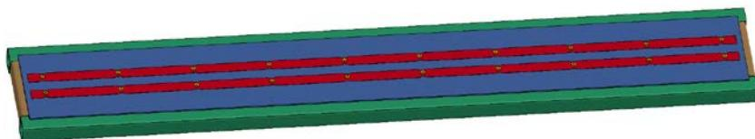
Fig.3: Adhesive layer placed between the top and base plates (in red).
