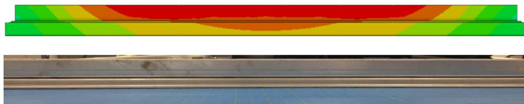
*Fig.15: Comparison of simulation and test: final shape of the plates (100 mm pitch) with a pre-cured adhesive layer.*
