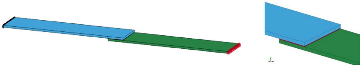
Fig.6: Simulation of the lap shear test in LS-DYNA.
