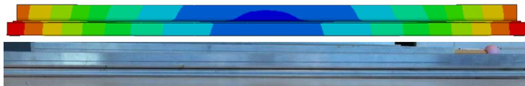
*Fig.14: Comparison of simulation and test: final shape of the plates (900 mm pitch) with a nominally pre-cured adhesive layer.*
