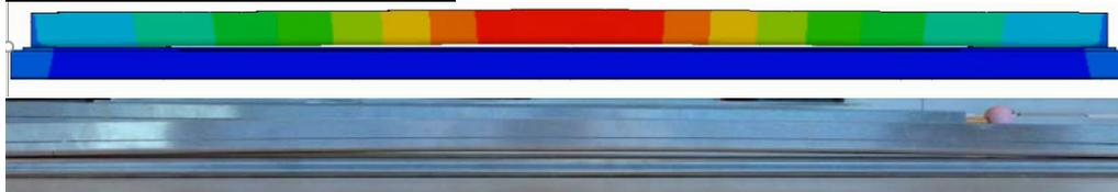
Fig. 13: Comparison of simulation and test: final shape of the plates with no adhesive layer.
