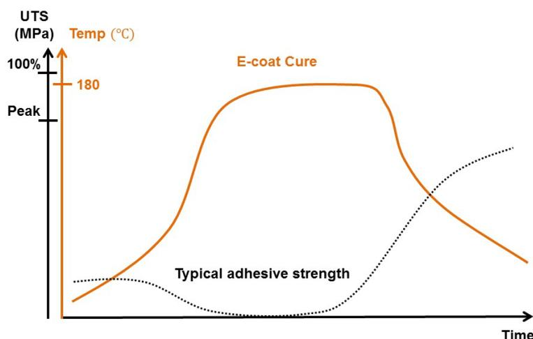
Fig.2: Temperature profile of the baking oven and the properties of the adhesives.
