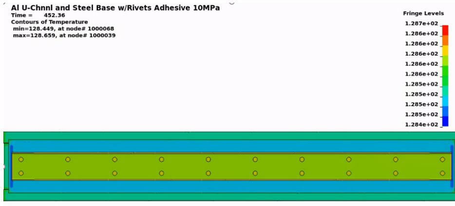
Fig.9: Temperature contour of the sandwich structure using a thermal-structural coupled analysis.
