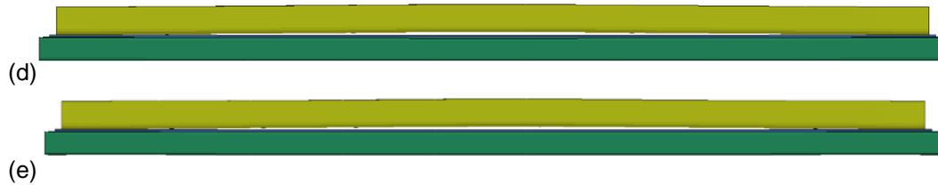
Fig. 11: Deformation of plates with no adhesives during the baking.
