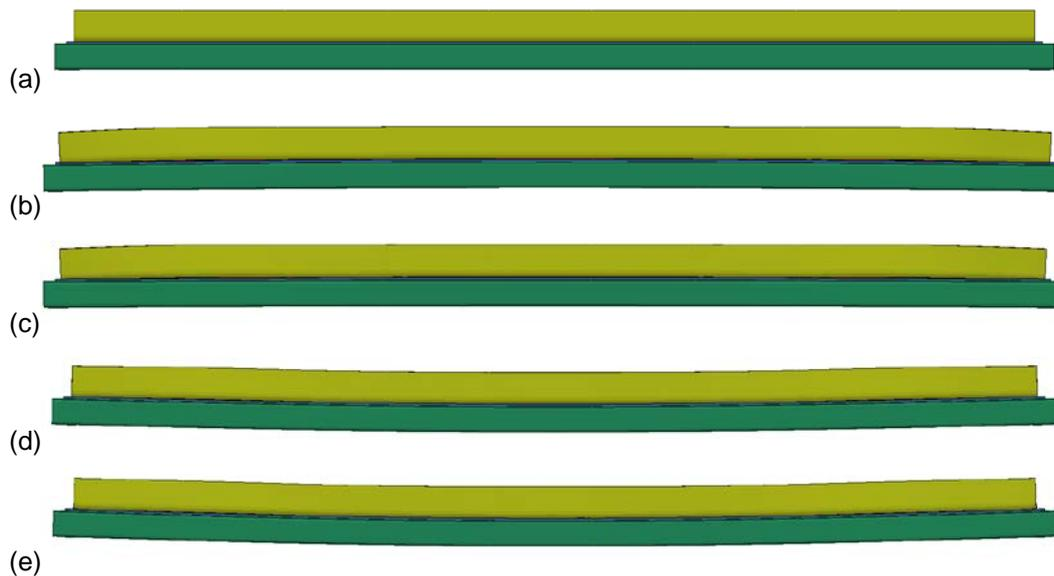
Fig. 12: Deformation of plates with adhesive during the baking process.
