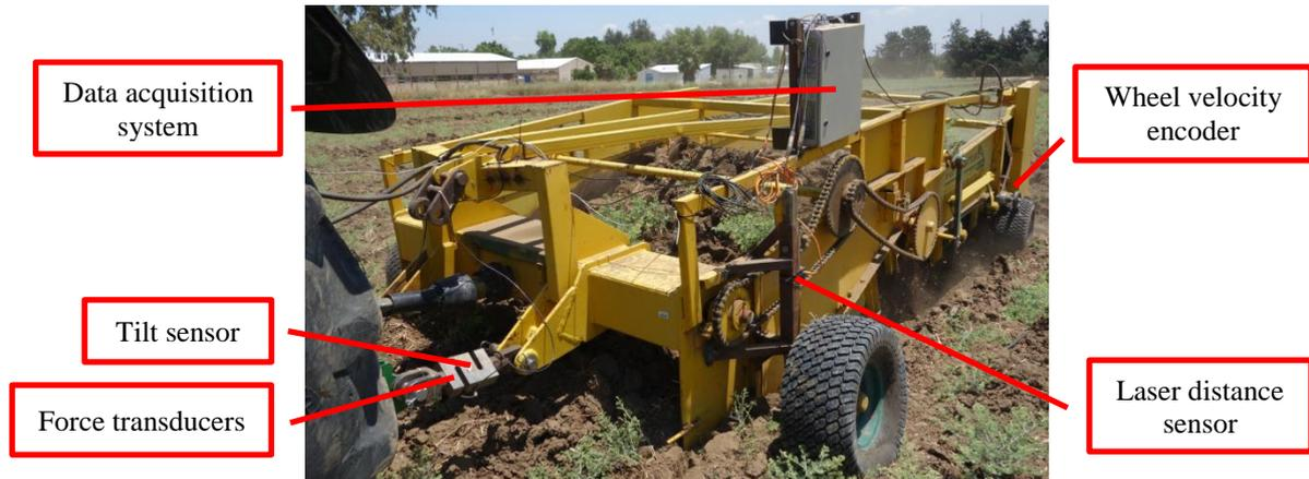
Fig.4: Acquisition system and sensors at the experiment.
