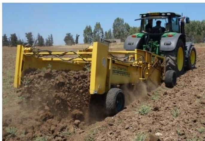
Fig.3: Full scale tillage machine field drag experiment.
