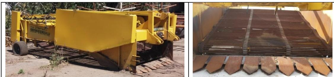
Fig. 1: Nutsedge pest control tillage machine.
