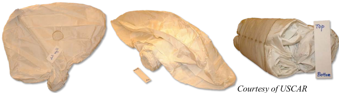
Fig.23: Photos of the PAB from USCAR research in unfolded, partly-folded and folded states
