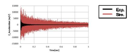
Fig.9: The acceleration result of drop test simulation without damping setting)
