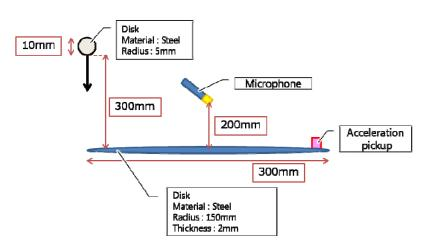
Fig.2: the image of drop test
