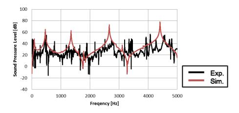
Fig.11: Acoustic analysis result compared with experiment data
