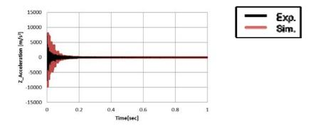
Fig.10: The acceleration result of drop test simulation with damping setting
