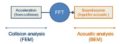
Fig.7: The Flow of Acoustic Analysis with Collision
