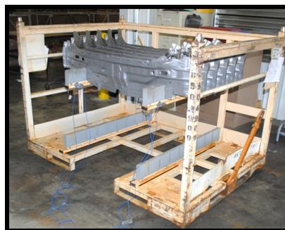
Fig.1: Photograph of the subject shipping cart shown with five automotive parts on top row and an empty bottom row.
