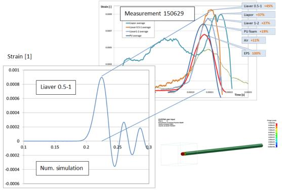
Figure 10: Comparison of numerically and experimentally found results of explosive load testing
