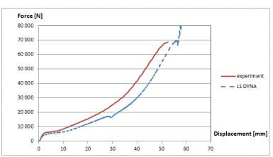
Figure 2: Comparison between numerically and experimentally found material behaviors (quasistatic compression)
