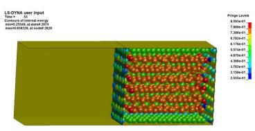
Figure 1: LS-DYNA simulation of quasistatic compression
