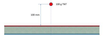
Figure 11: Blast load experiment setup
