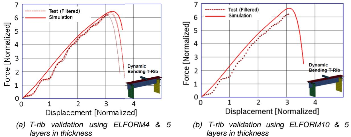
Fig.4: Validation on specimen level simulation and test, using different element formulations: ELFORM4 (a), ELFORM10 (b).
