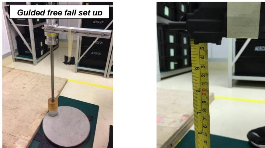
Fig.7: Guided free fall test set up.
