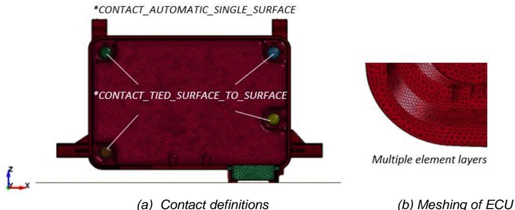
Fig.6: Finite element model of the ECU (a) tied contacts for screws and automatic single surface contact overall; (b) in thickness direction multiple layers of tetrahedron elements, ELFORM 4.
