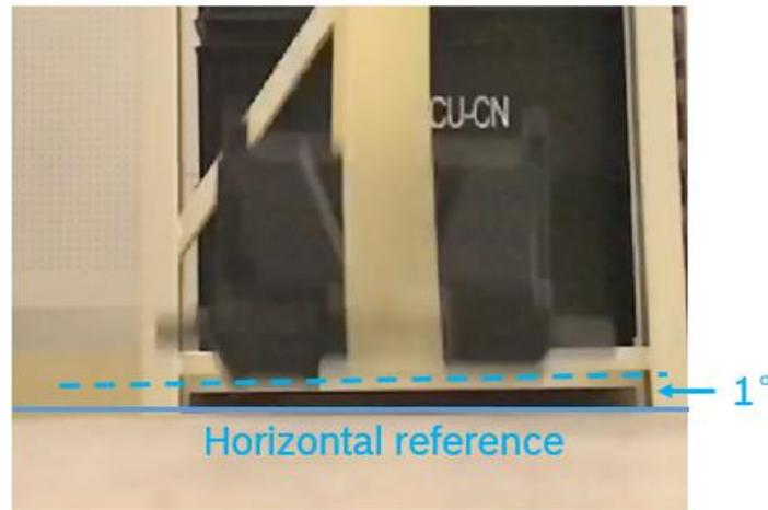
Fig.10: Representative example of impacting angle recorded by high speed camera.
