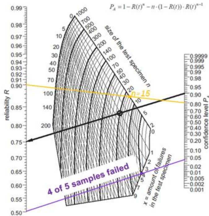
Fig.11: Larson nomogram (based on diagram from [10]), relationship between number of total samples, number of passing samples, reliability and confidence level.
