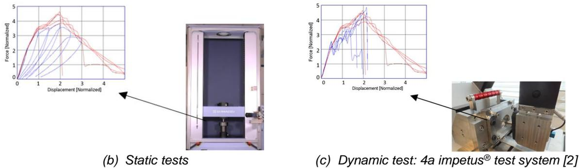
Fig.3: Puncture test with simulation model (a) and test set up and measurement results (b), (c) [4]; each test is repeated 5 times; static results shown in different colors are of different loads; dynamic results shown in different colors are of different puncture velocities.
