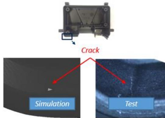
Fig.8: Crack detected at housing corner, same location in simulation as in guided free fall experiment.
