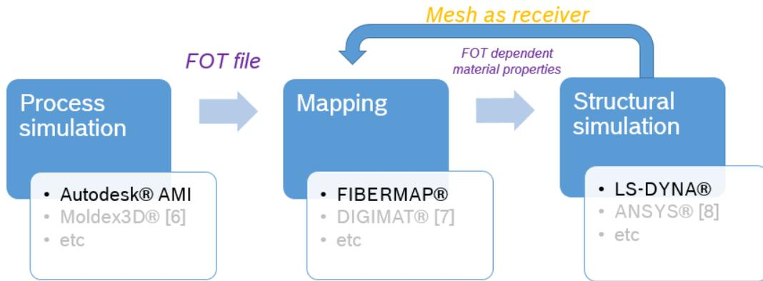
Fig.5: General workflow for the integrative simulation toolchain.
