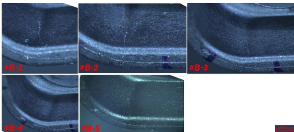
Fig.9: Result of visual inspection under microscope of test series B samples after drop.
