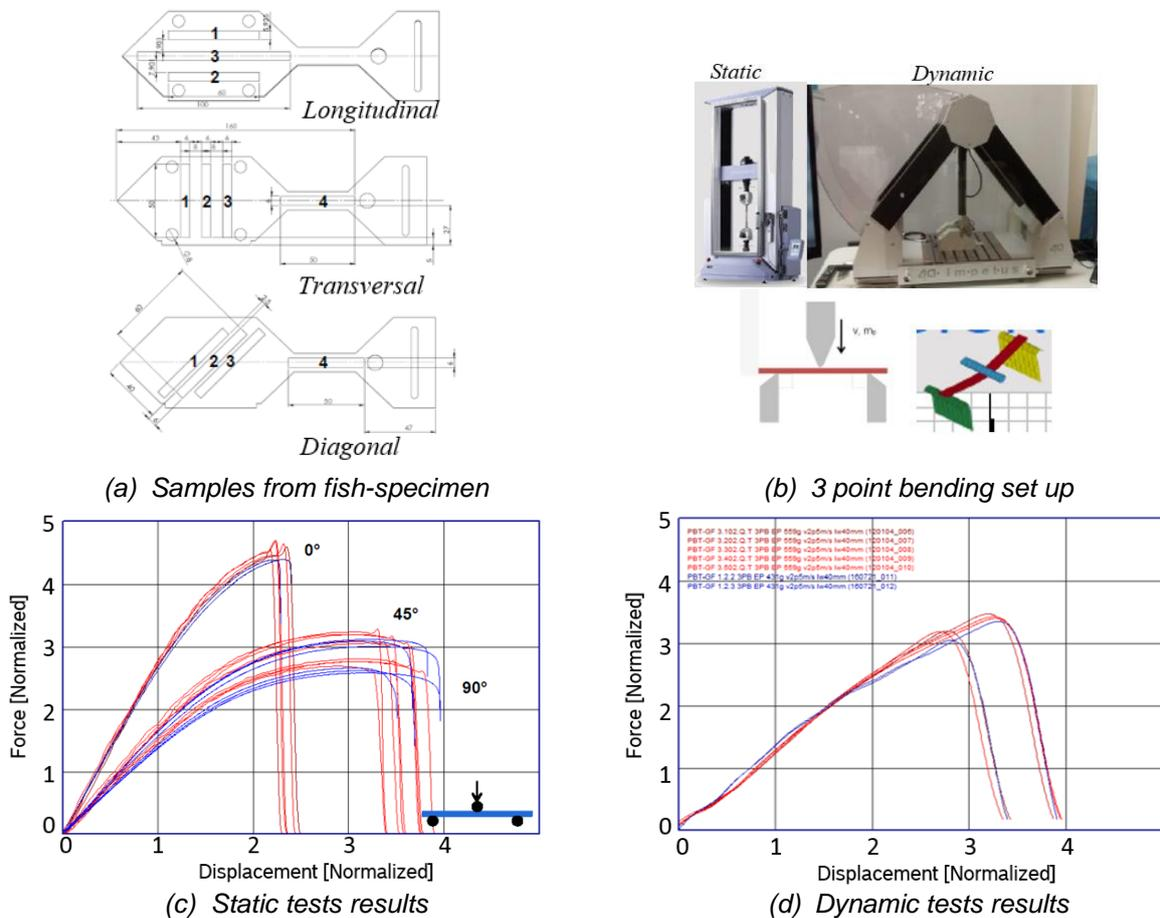
Fig.2: 3 point bending test with specimen (a), set up (b) and results overview (c), (d) [4]; each test is repeated 5 times; dynamic test results are of diagonal specimen; test results in red are from samples tested in 2016, test results in blue are from samples tested in 2012 – only approximately 5% scattering/difference is observed.
