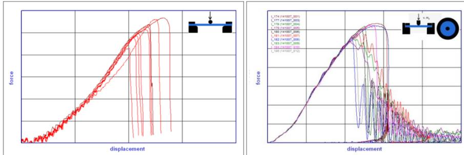
Fig.3: Force-displacement curves for clamped 3-point-bending (left) and dynamic puncture test (right) for a ductile material; failure occurs for all test specimens [2]
