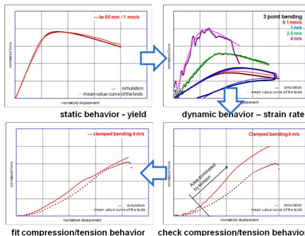
Fig.7: Improved workflow in 4a impetus to determine a complex yield surface [6]
