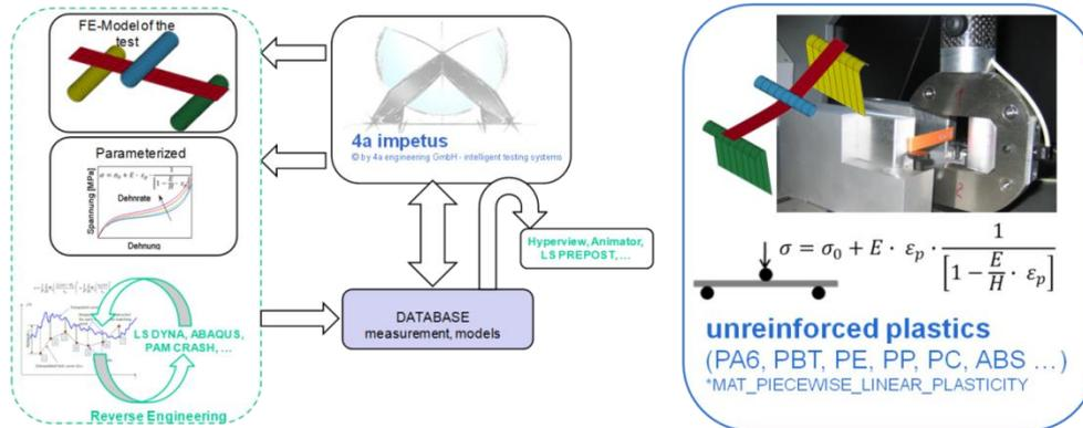
Fig.5: Material characterization by reverse engineering using the 4a impetus process [5]
