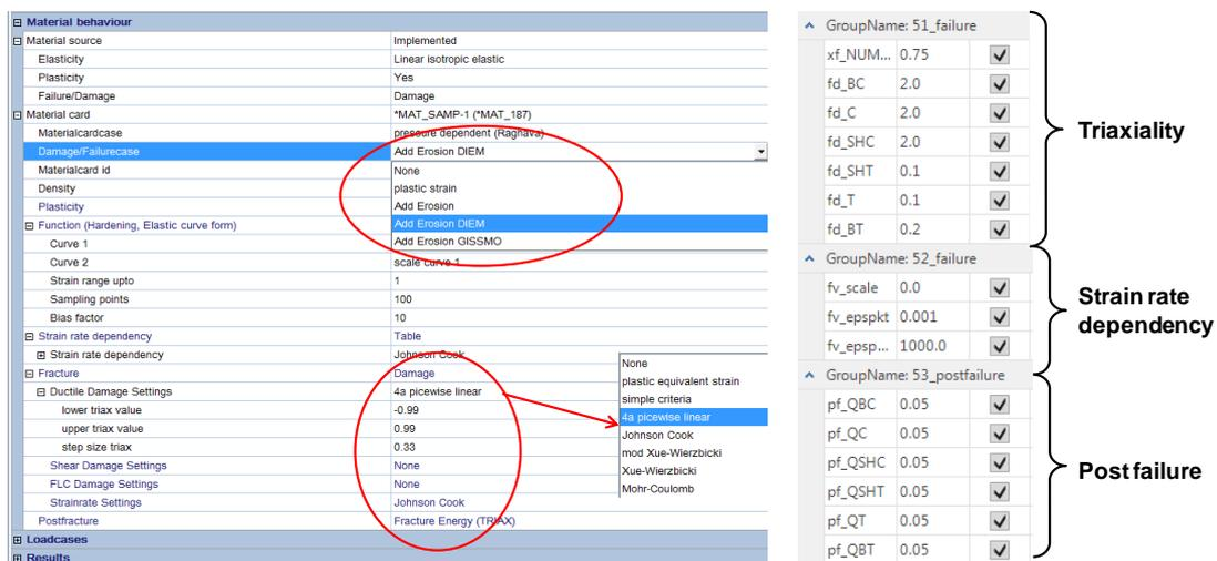
Fig.11: Modeling failure in 4a impetus (left); according design variables for the chosen failure model (right) [3]
