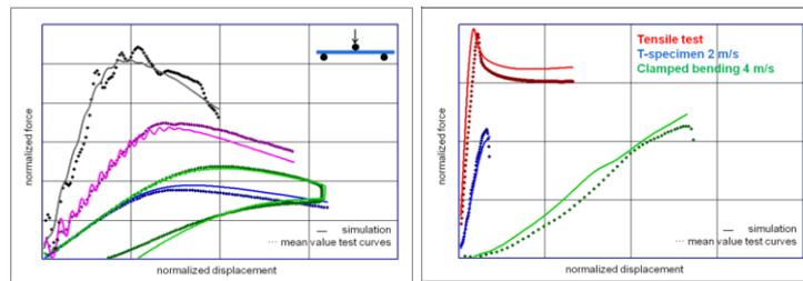
Fig.8: Result of the reverse engineering process for 3-point bending test curves at different velocities (left) and validation of the material card for further load cases (tensile test, clamped 3-point bending test and T-specimen test) using **\*MAT\_187** [6]
