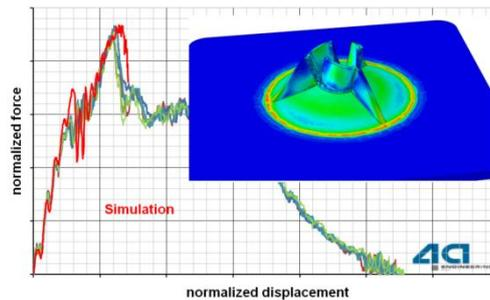
Fig.10: Comparison of test and simulation results for a part characterized by a complex material model [6]
