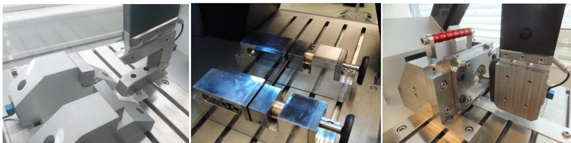
Fig.2: Dynamic bending test (left); dynamic clamped bending test (middle); dynamic puncture test (right) [1]
