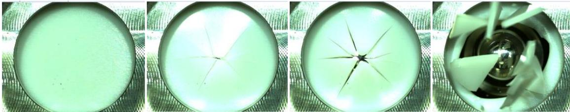
Fig.4: High speed pictures of the dynamic puncture test of a POM at different time steps [3]
