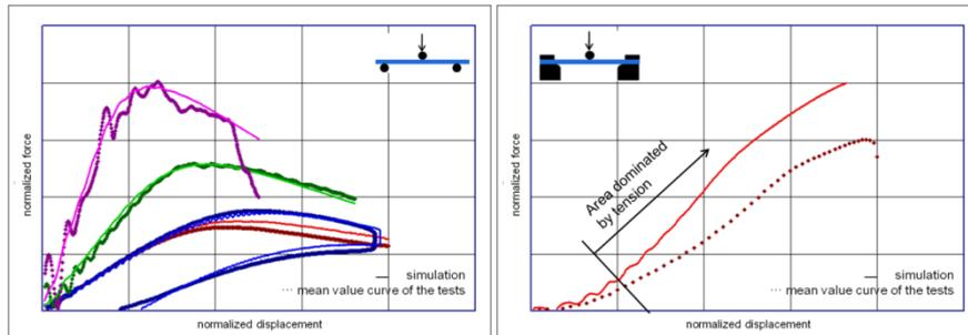
Fig.6: left - Describing the material behavior using **\*MAT\_024** for bending tests at different velocities; test and simulation curves match very well.
