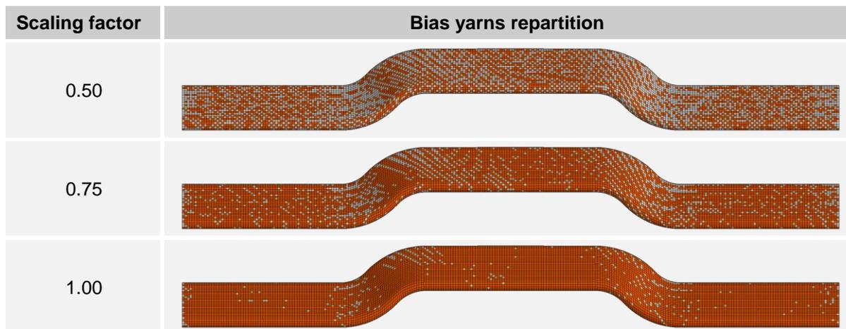
Fig.8: Repartition of the braid yarns (in orange) after mapping depending on the scaling factor
