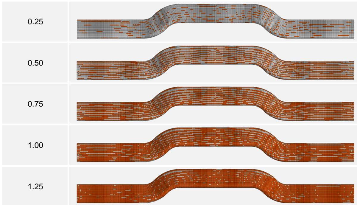
Fig.7: Repartition of the axial yarns (in orange) after mapping depending on the scaling factor
