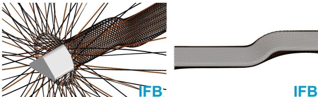
Fig.3: Braiding simulation (left) and view of the predicted fibre architecture (right) on the example of a generic component
