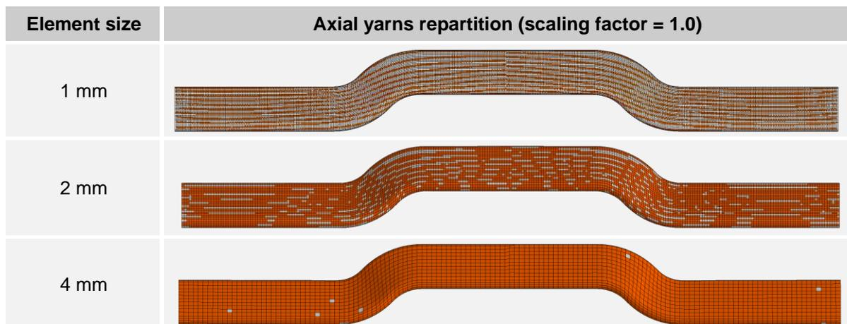
Fig.9: Repartition of the braid yarns (in orange) after mapping depending on the element length
