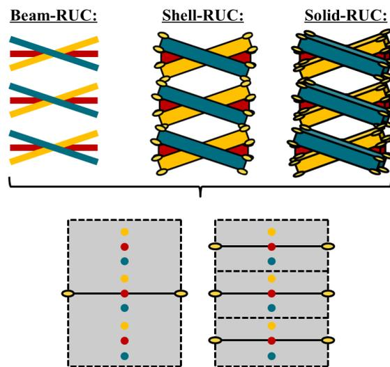
Fig.4: Mapping procedure within ENVYO for different input and target meshes
