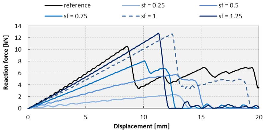
Fig.10: Force-displacement diagrams for different scaling factor values in comparison with the reference approach
