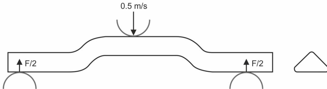
Fig.6: Testing conditions for the generic component under three-point bending
