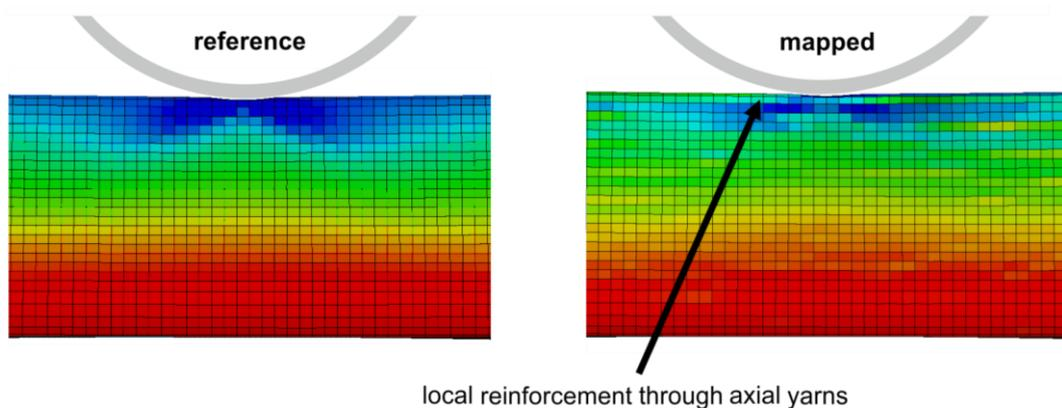
Fig.11: Local influence of the axial yarns on the axial stress field (fibre compression)
