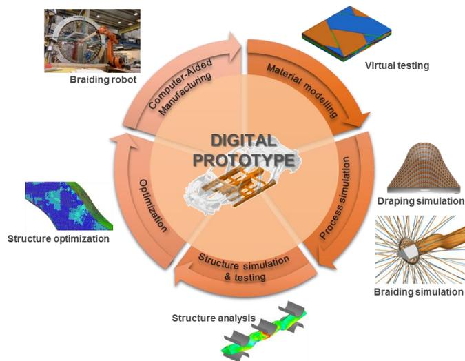
Fig.2: Numerical process chain developed in the project DigitPro
