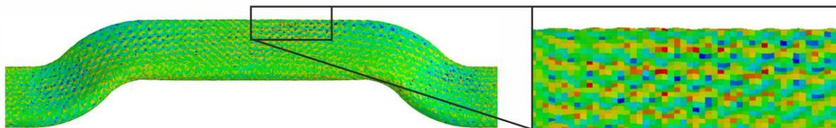
Fig.5: Variable thickness and resulting surface waviness in the generic component after the mapping of the braiding simulation
