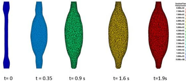
Fig.9: Feasibility Analysis – pressure distribution during balloon deployment
