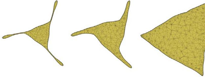
Fig.13: Fluid mesh development during balloon expansion
