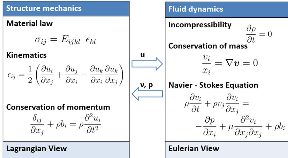
Fig.3: Overview of the governing equations of FSI
