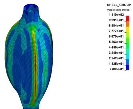
Fig.11: Van Mises Stress distribution during balloon deployment
