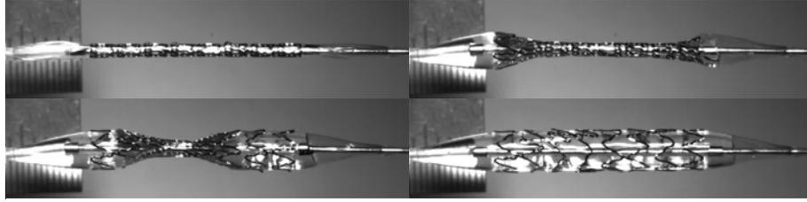
Fig. 1: Slow motion track of the deployment of a balloon expandable stent demonstrating the non-symmetrical dog-bone effect
