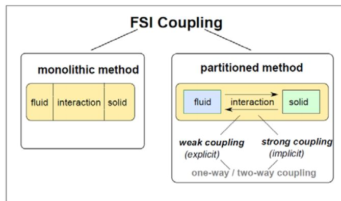
Fig.4: Overview of the FSI modelling approaches
