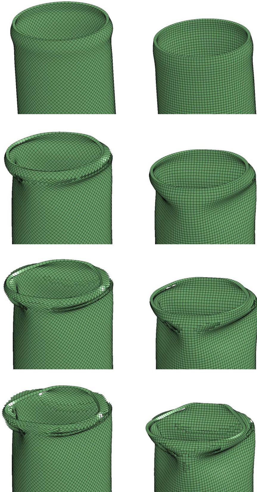
*Fig.6: Also the element orientation has some influence on the predicted deformation mode.*
