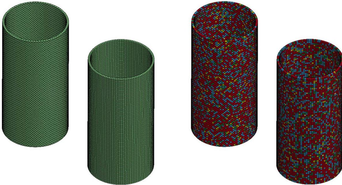
Shell elements to capture the surface strain
