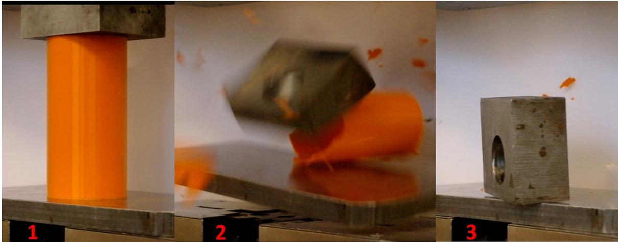
Fig.2: Some pictures from quasi-static compression of a 3D-printed tube with  $L=2D=60T$ .
