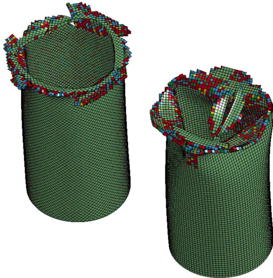
Fig.7: *FEM seems to delete too many elements instead of fracture between segments.*
