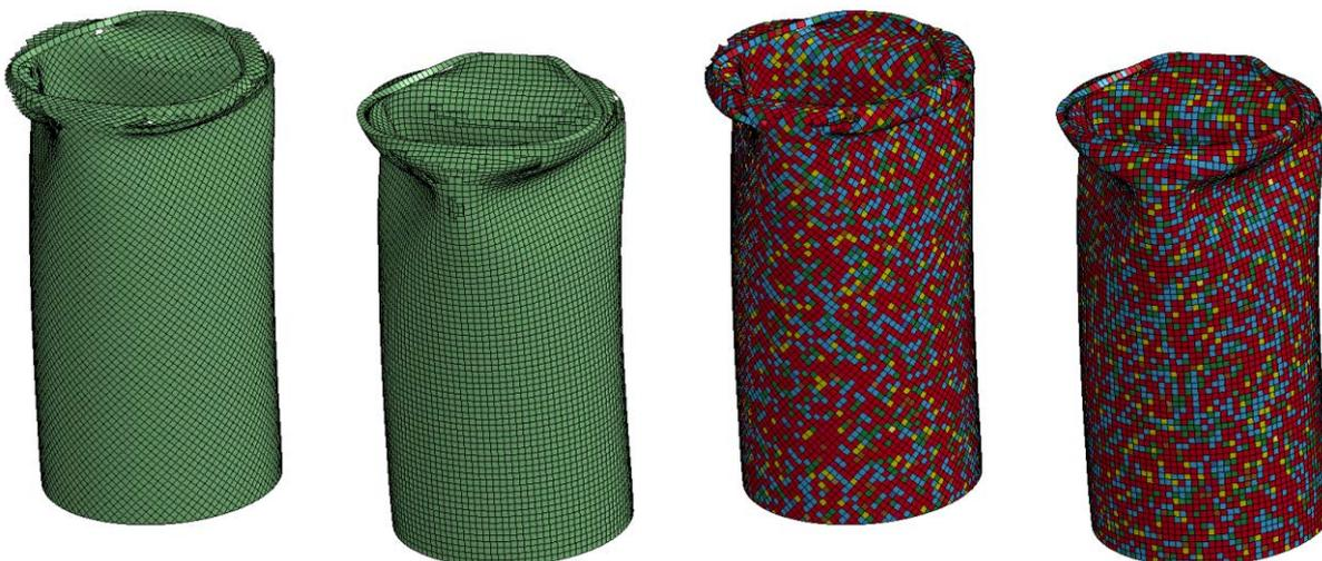
Deleted surface elements define the cracks
