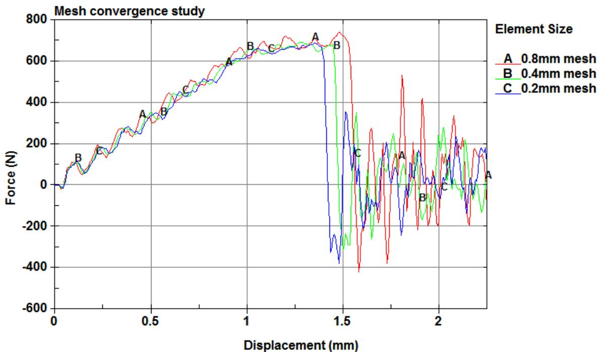
Figure 8 Comparison of force-deflection curves for various mesh densities
