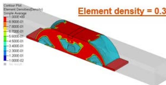
Figure 1 Optimized topology with threshold element density = 0.3
