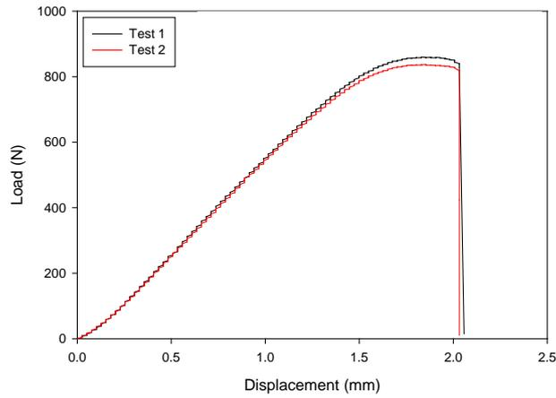
**Figure 9 Force vs. deflection curves form physical tests for topology optimized geometry**
