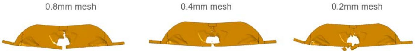
Figure 7 Comparison of failure patterns for various mesh densities
