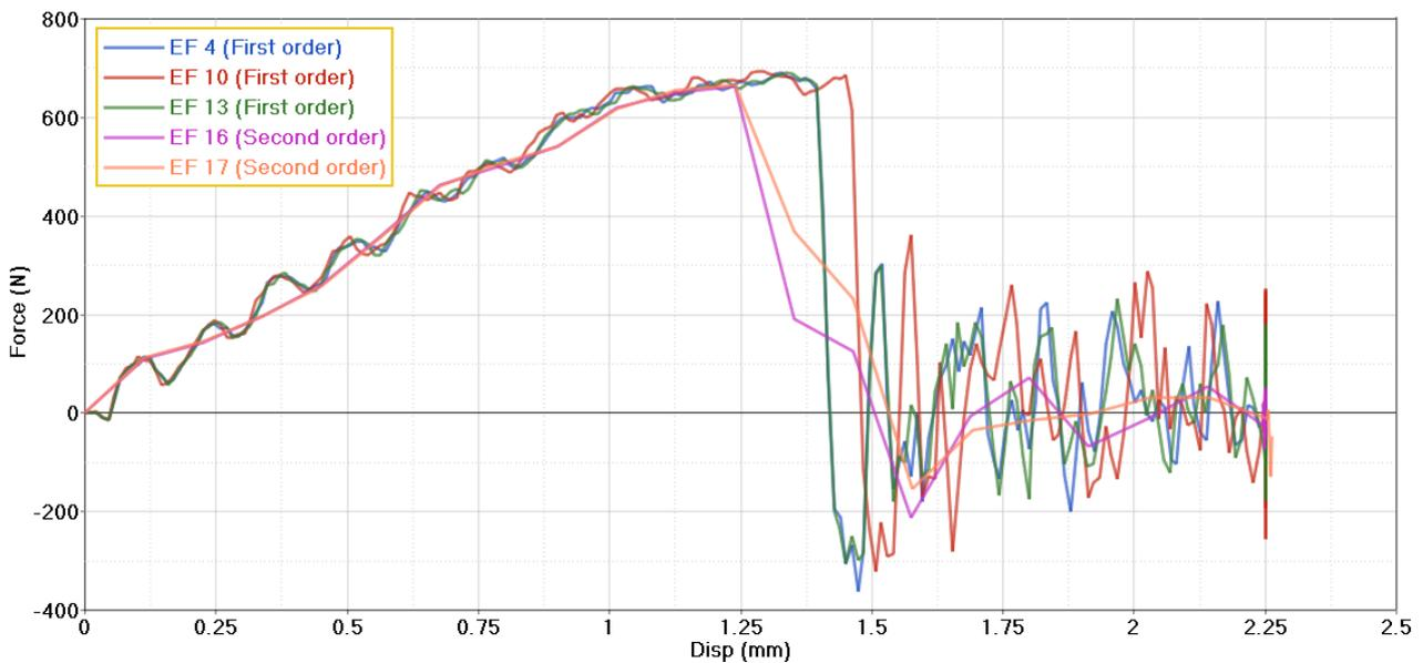
**Figure 6 Comparison of force vs. deflection curves for different element formulations**
