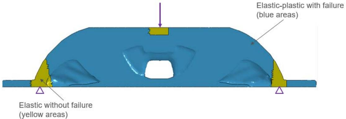
Figure 4 Model Set-up
