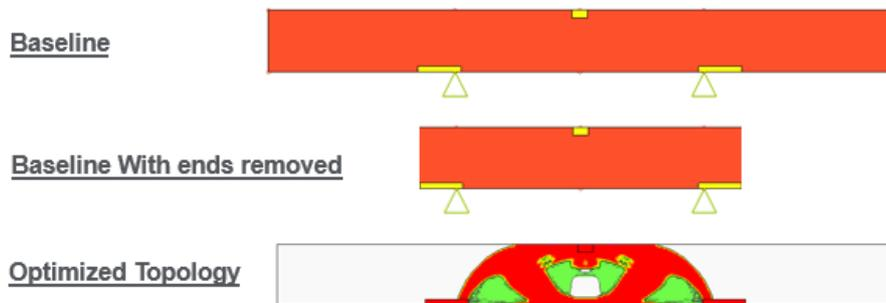
**Figure 3 Illustration of lightweight configuration with optimized topology**
