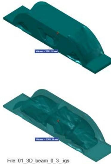
**Figure 2 Internal geometrical complexities after topology optimization**
