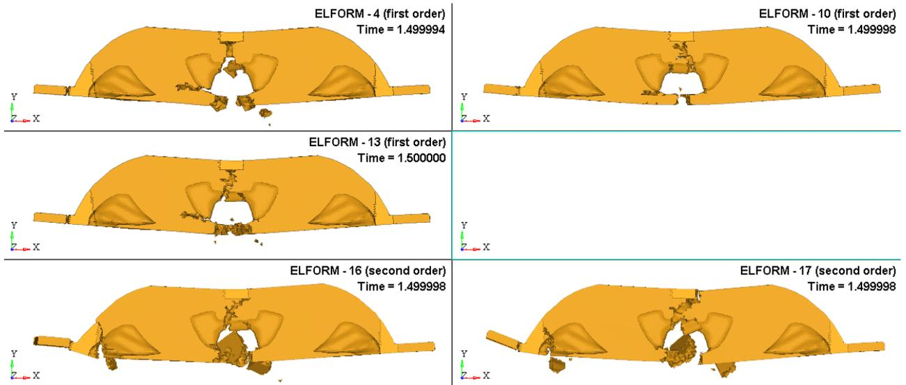
**Figure 5 Comparison of failure patterns for different element formulations**
