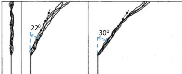
Fig. 11. Experimental crack paths under impaction [28]
