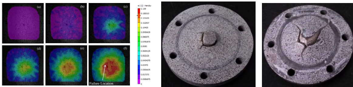
Fig.9: DIC images and specimens tested in the dynamic punch test.
