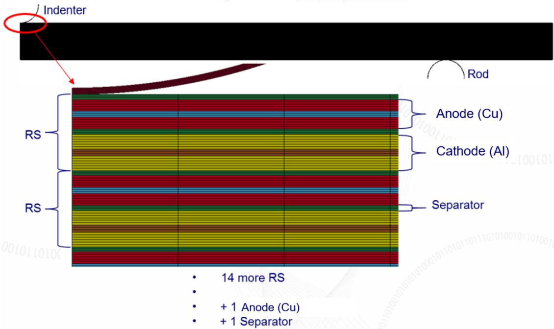
Fig.4: Mesh of the 3-points bending simulation on the complete cell for the element aspect ratio with element formulation solid -1 (particular case of the ratio aspect = 20)
