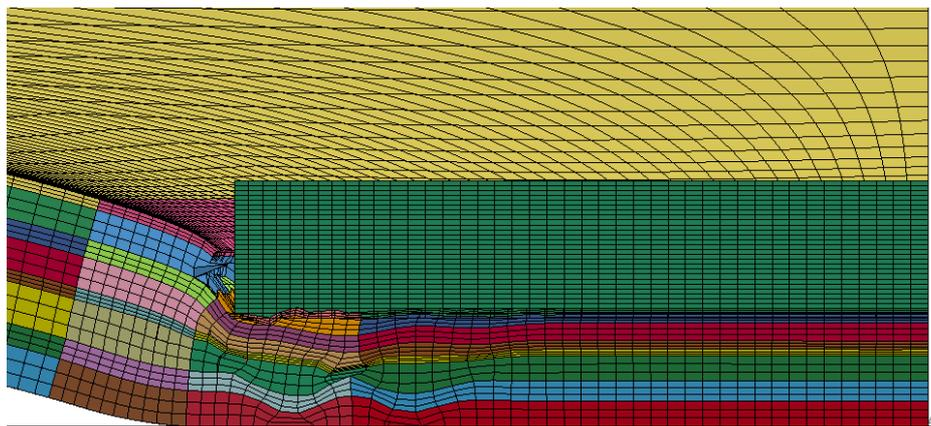
Fig.10: Deformed shape of the model at the final stage of the indentation before error termination. Side view
