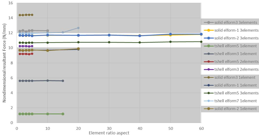
Fig.2: Element aspect ratio study on 3-points bending simulation. Resultant force comparison between element formulations
