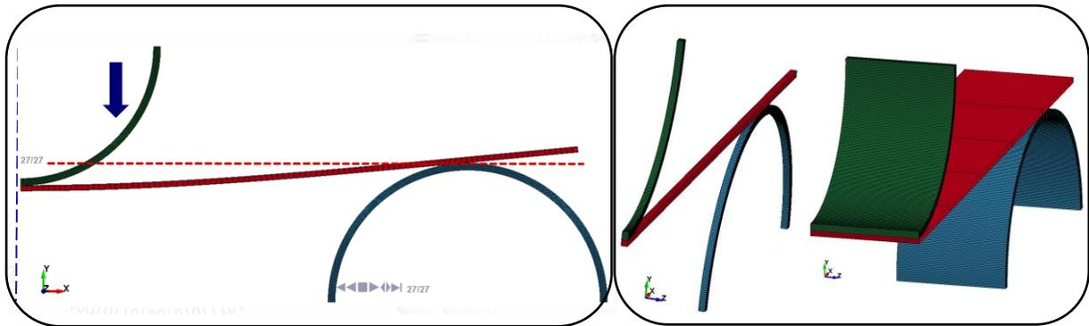
Fig. 1: Mesh of the 3-points bending simulation for the finite element formulation study (particular case with one element through the thickness). Side view on the left. On the right, the aspect ratio is highlighted with the width difference between models)
