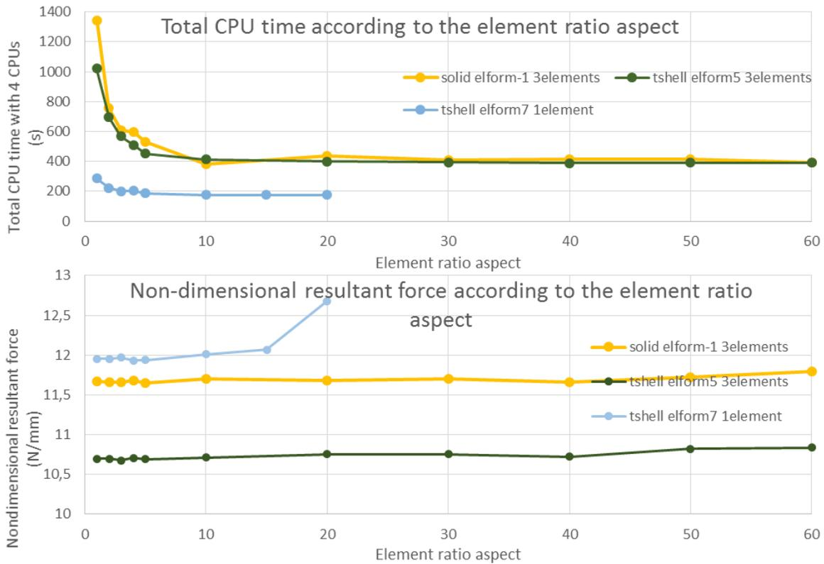
Fig.3: Three finalist element formulation after sorting out those which gave unsatisfying results on 3-points bending simulation. Total CPU time and resultant force over the element aspect ratio
