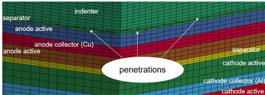
Fig.9: Highlighting of penetrations in local indentation study
