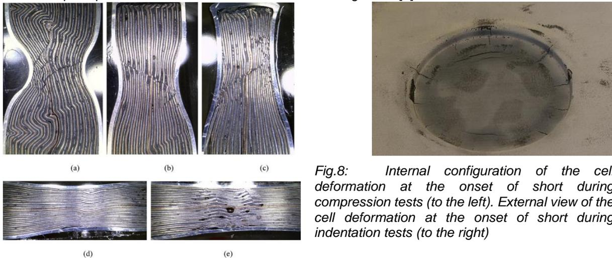
Fig.8: Internal configuration of the cell deformation at the onset of short during compression tests (to the left). External view of the cell deformation at the onset of short during indentation tests (to the right)
