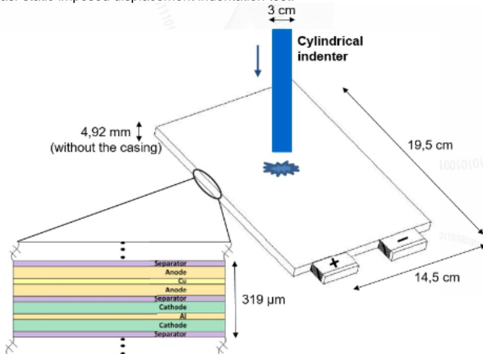
Fig.6: Schematic representation and dimensions of Ford experiment indentation tests
