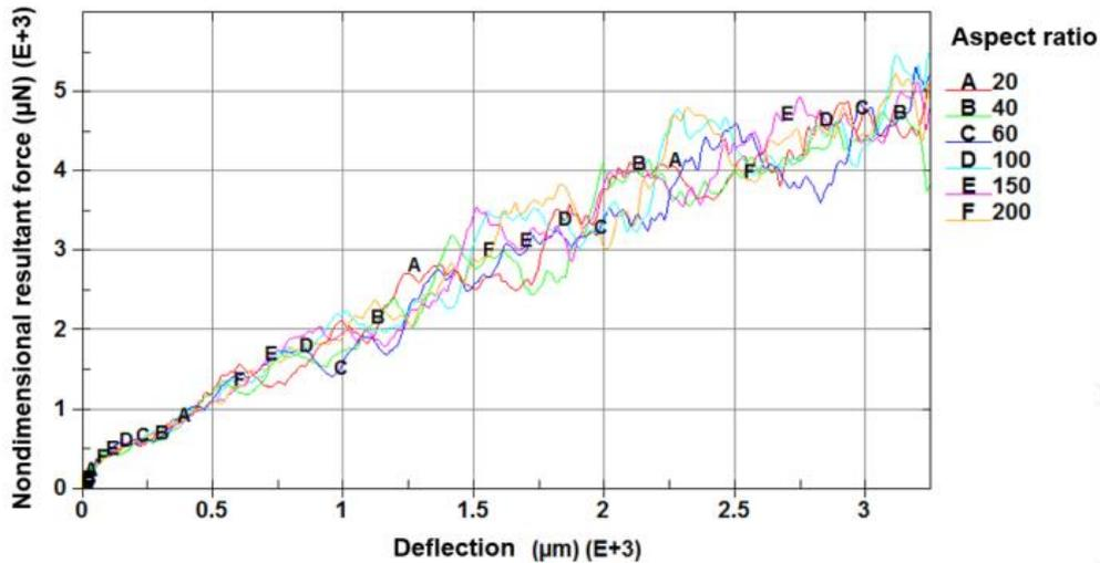
Fig.5: 15 points floating average on the structural response of the complete cell with one element through the width on the 3-points bending simulation
