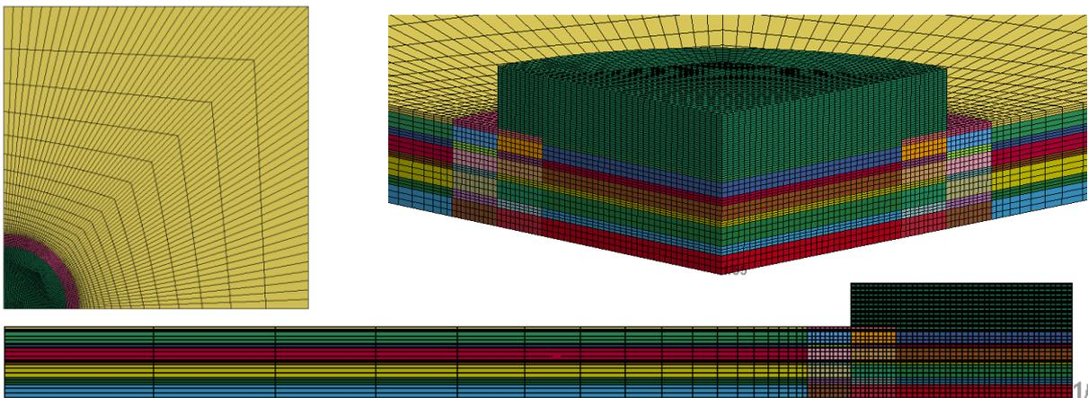
Fig.7: Three different views of the mesh used for the indentation study
