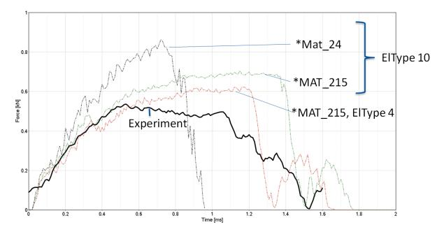
Fig.8: Force-time curves of the drop tower test on the component from experiment and simulation with different material models and element types.
