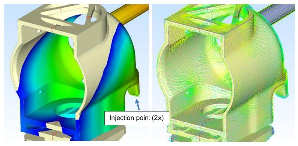
Fig.6: Pictures of the mould flow simulation results, showing the injection point, the melt front and the surface fibre orientation.
