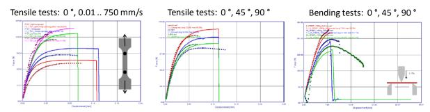
Fig.2: Selection of test data for various load cases and loading rates with the simulation curves of the \*MAT\_215 material model, which was fitted with 4a-fibermap software. The dotted curves show the force-displacement curves of the experimental test, the simulated curves are represented by the solid lines.
