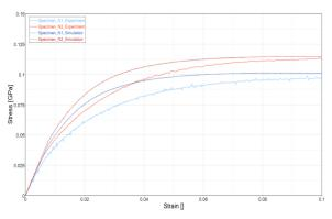
*Fig.5:* Stress-strain curves of the fibre-orientation specimens with simulated data with the modified material model accounting for the reduced fibre aspect ratio and the low strain rate.
