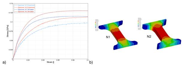
Fig.4: a) Stress–strain curves and b) simulated von-Mises stress fringe plots of fibre-orientation specimens during tensile testing. The formation of a mid-layer in specimen N1 leads to a reduced stress level in the core of the sample.
