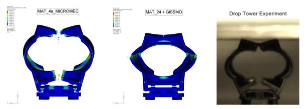
Fig.7: Failure mode of **\*MAT\_4a\_MICROMEC** model considering local anisotropies and isotropic **\*MAT\_024** Model in comparison with experimental drop tower experiment.
