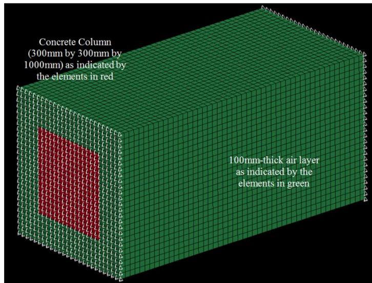
Fig.5: Screenshot of model showing 2 node sets at either end where one end is fixed in displacement in the axial direction, and the other is applying the axial load via velocity to the nodes
