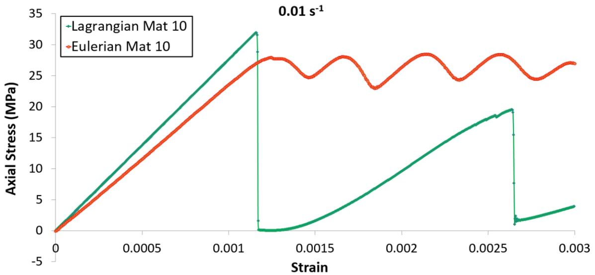
Fig.7: Axial stress-strain curve at strain rate of 0.01 per second (\*MAT\_010)
