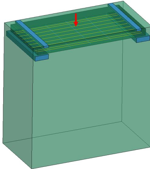
*Fig.11: Setup of the blast loaded reinforced concrete slab*
