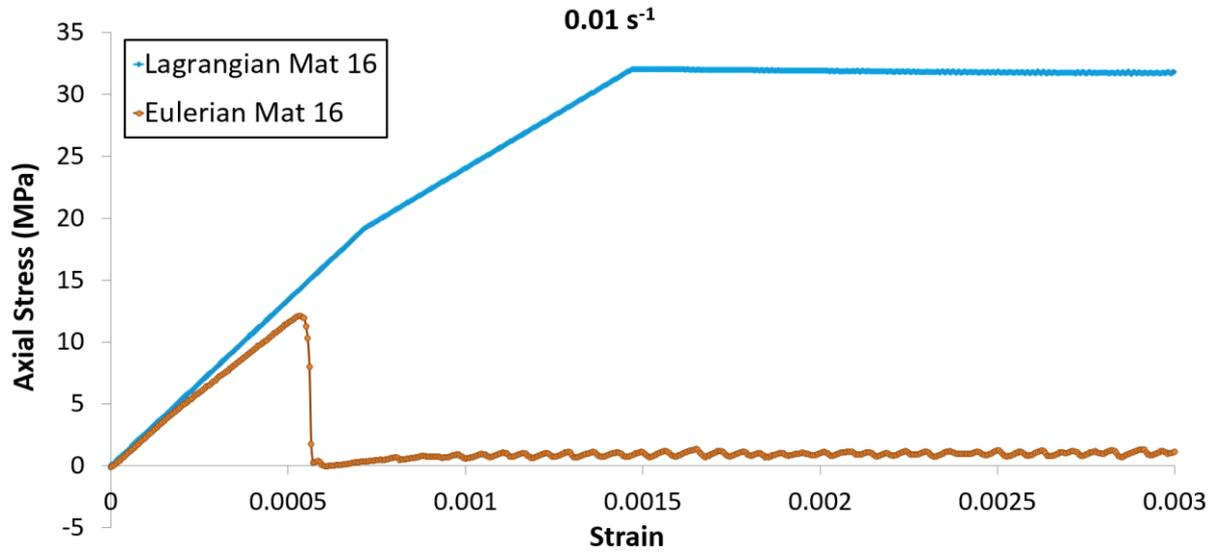
Fig.8: Axial stress-strain curve at strain rate of 0.01 per second (\*MAT\_016)
