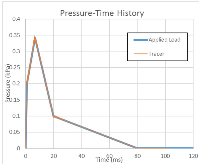
Fig.13: Pressure time history recorded by tracer compared to applied load
