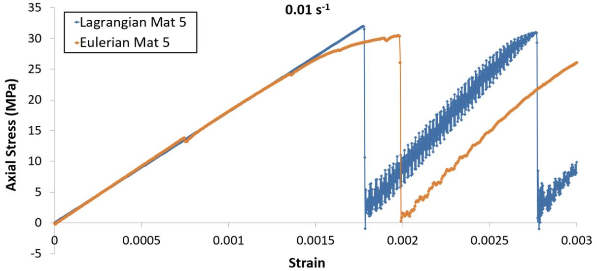
Fig.6: Axial stress-strain curve at strain rate of 0.01 per second (\*MAT\_005)
