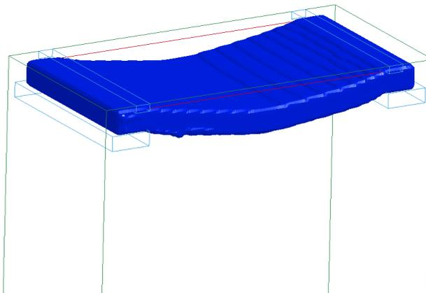
Fig.16: Deflection of the ALE reinforced concrete slab
