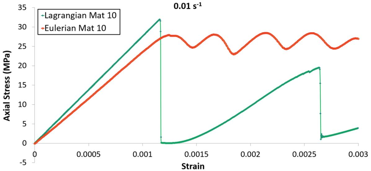
Fig.7: Axial stress-strain curve at strain rate of 0.01 per second (\*MAT\_010)
