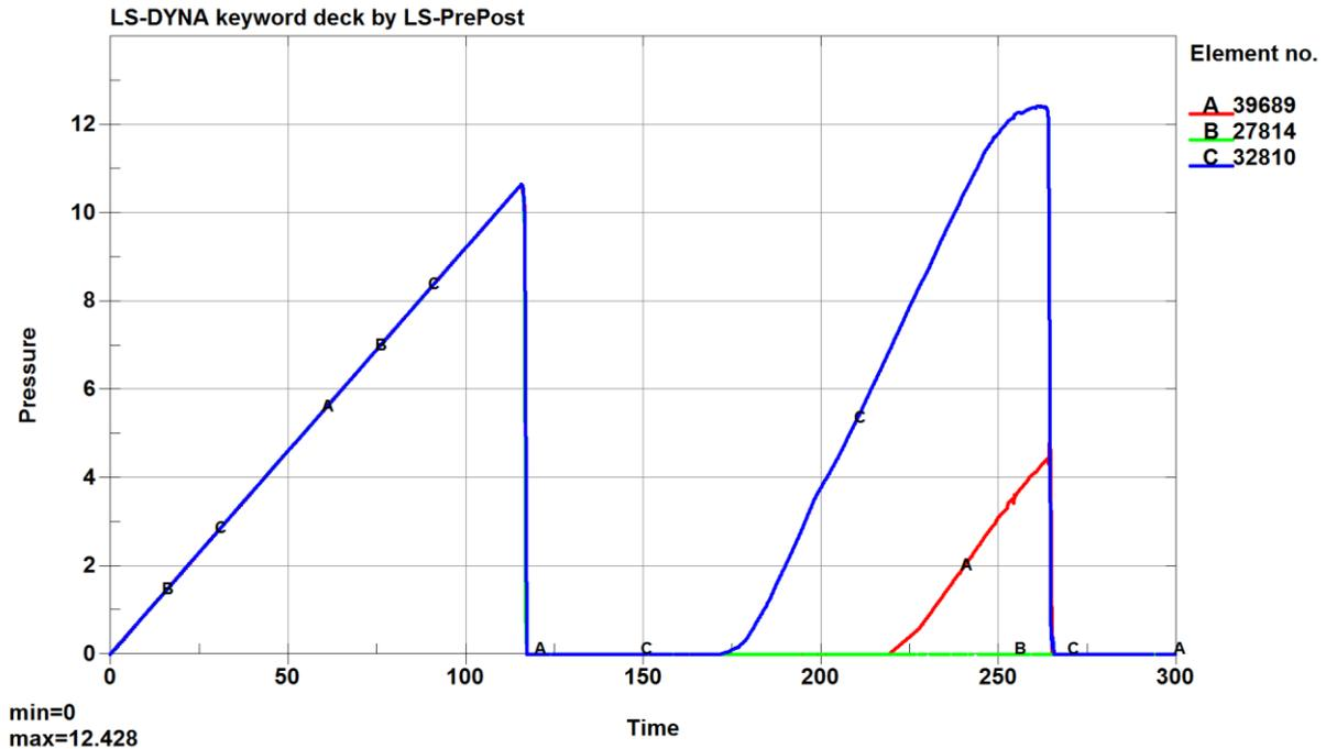
Fig.10: Mean stress-time curve (\*MAT\_010)
