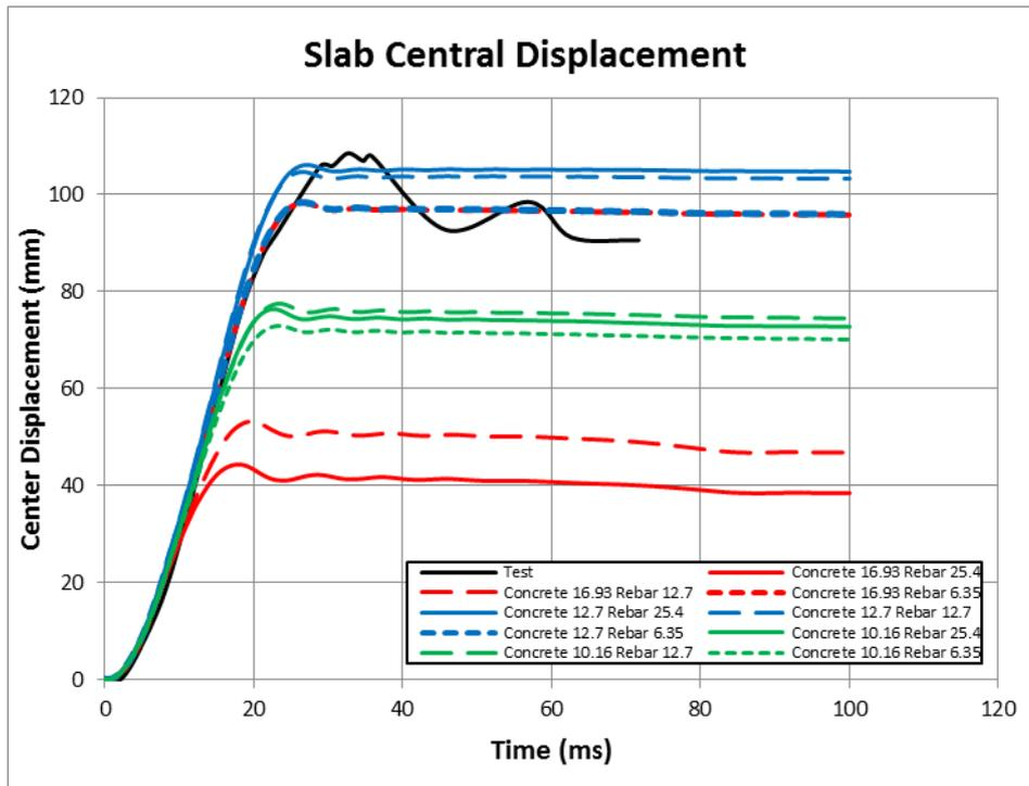
Fig.15: Slab central displacement for ALE reinforced concrete slab
