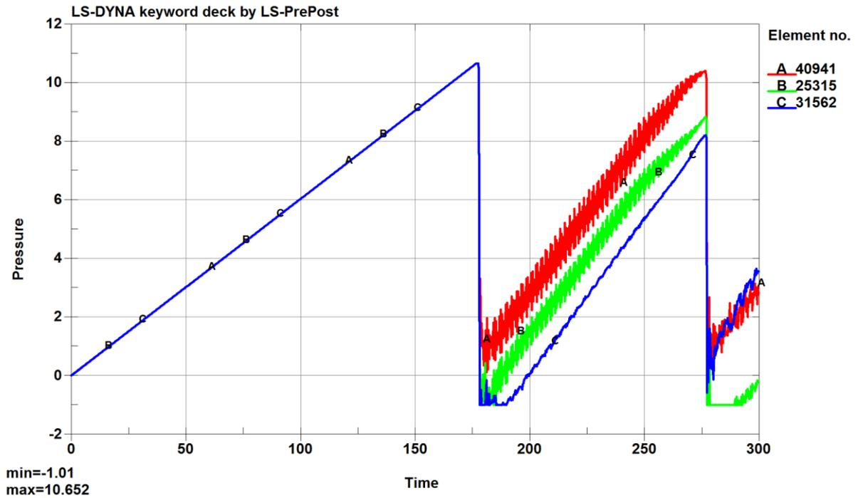
Fig.9: Mean stress-time curve (\*MAT\_005)
