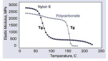
Fig.1: Modulus vs. temperature plot for unreinforced nylon 6 (semi-crystalline) and PC (amorphous). The materil properties change significantly with the temperature and this will affect the mechanical response and consequently the flow around it.
