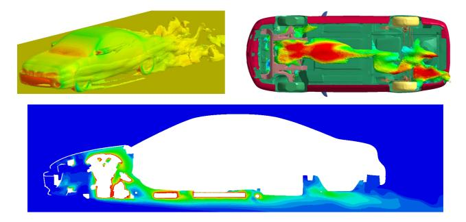
*Fig.3:* Results for the aerodynamics benchmark on a GMC vehicle. Top left shows the iso-surface of velocity, top right is iso-surface a fluid temperature and bottom is a cutplane with iso-contours of temperature showing the higher tempreature around the engine block and exahust.
