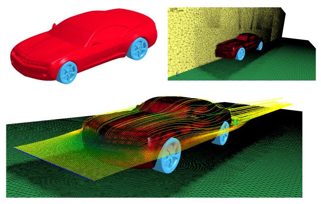
Fig.4: CFD analysis of a vehicle which will be used for FSI simulation.
