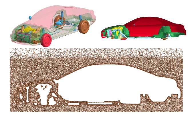
*Fig.2:* Geometry and cut plane of a GM Pontiac model used for benchmarking the CFD solver and coupling it to the thermal analysis.
