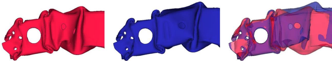
Fig.3: Scatter mode deformation shapes for left longitudinal rail
