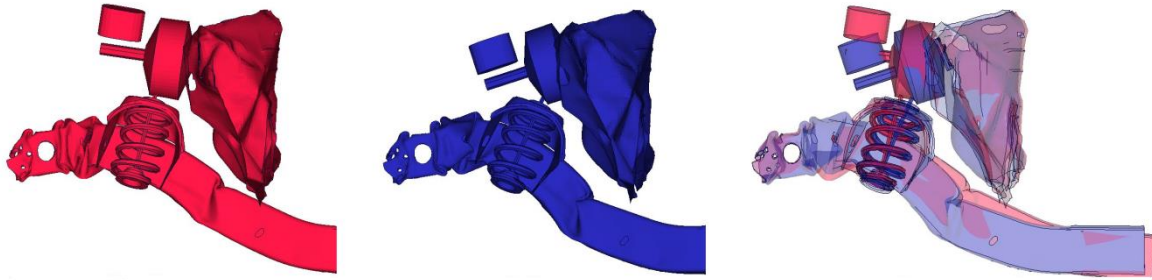
Fig.2: Scatter mode deformation shapes for shock absorber – brake unit interaction
