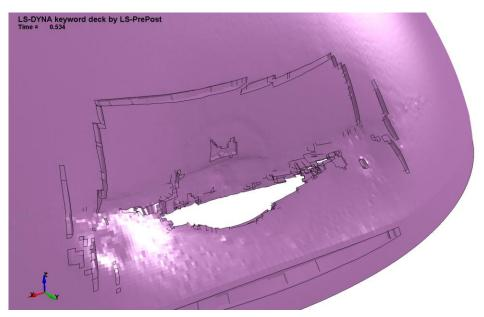
Fig.12: Perforation of the dome from the analysis with "rigid mass" model
