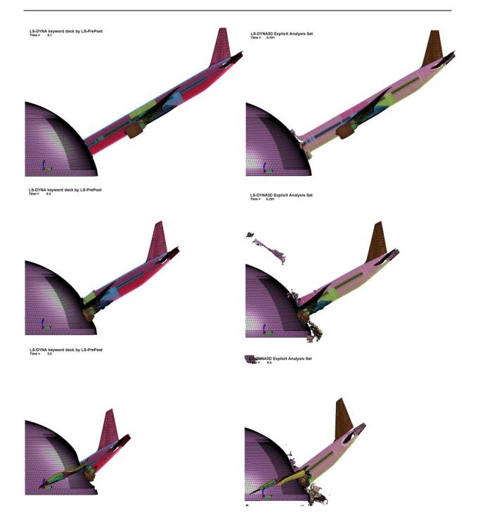
*Fig.11:* Impact of the aircraft with "rigid model" (left) and SPH model (right, SPH particles are not shown)
