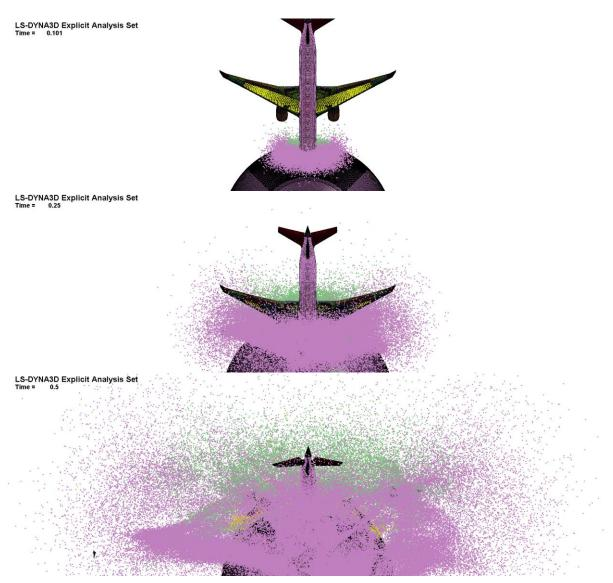
Fig.14: Debris cloud at different stages of the analysis with SPH mass model
