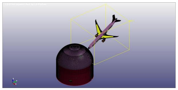
Fig.4: Box for the SPH approximation
