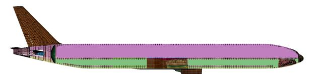
Fig.2: Position of the SPH corresponding to passengers, luggage and cargo
