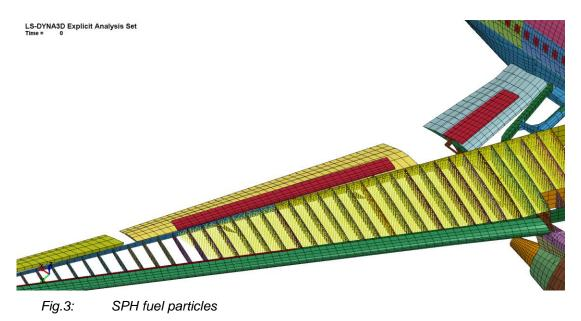
Figure 2 shows the position of the SPH corresponding to payload in the aircraft. The position of the SPH fuel particles in the wing of the aircraft is shown in Figure 3.
