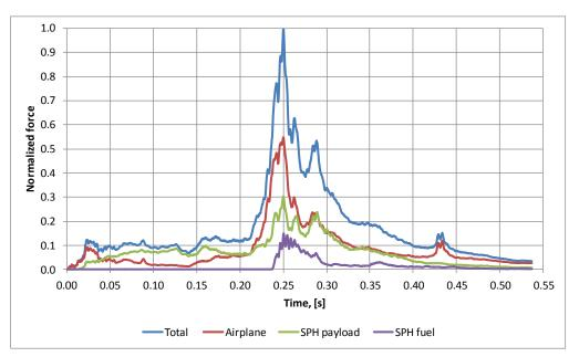
Fig.8: Resultant contact force form the analysis with SPH model of the non-structural mass
