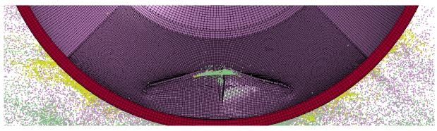
Fig. 15: Penetrating SPH into the containment structure, bottom-up view
