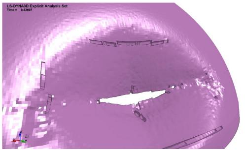
Fig.13: Perforation of the dome from the analysis with SPH model
