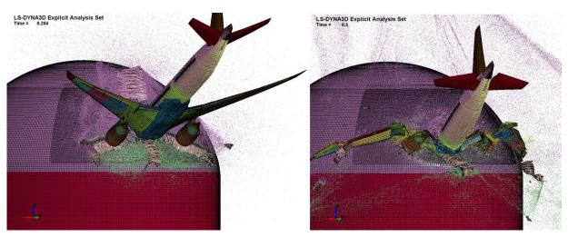
Fig.6: Impact at the concrete containment with SPH model
