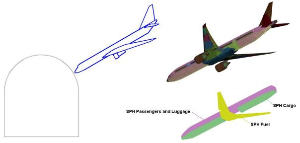
Fig.1: Impact configuration (left) and FE model of the aircraft (right)
