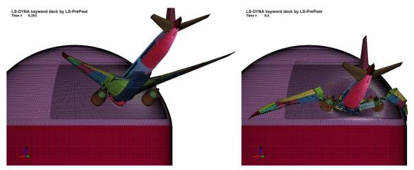
Fig.5: Impact at the containment with "rigid mass" model
