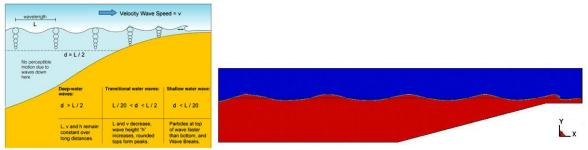
(a) wave type (b) wave simulation response behavior Fig. 19: Wave type and wave simulation response behavior according to water depth
