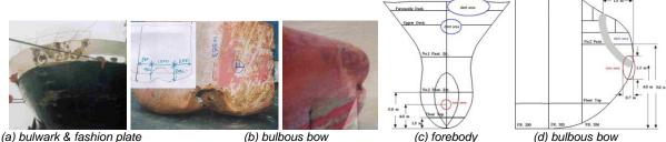
Fig. 30: Collision damage configurations and schematic damage drawings of striking ship
