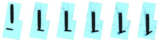
Fig. 11: Overall view of response behavior of full-scale collision simulation using FSI analysis technique
