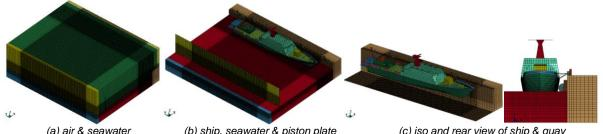
(a) air & seawater (b) ship, seawater & piston plate (c) iso and rear view of ship & quay Fig. 20: F.E. mesh configuration of quay mooring model of ship including air and vertical dock fenders, rope using FSI analysis technique
