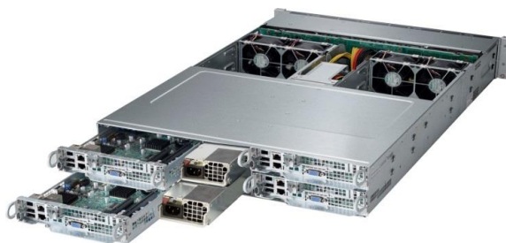
Fig.1: Overhead View of SGI Rackable Server with the Top Cover Removed
