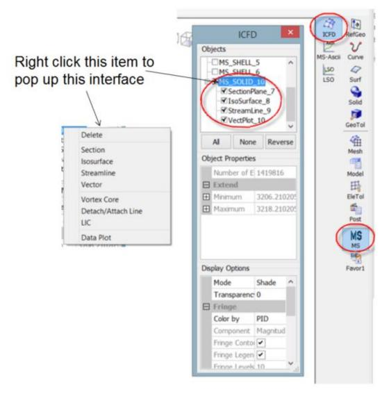
Fig.5: Interfaces for the new ICFD post-processing
