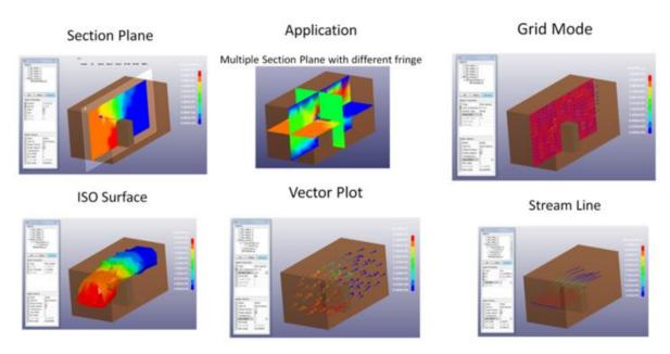
Fig.4: Different rendering options for the ICFD post-processing
