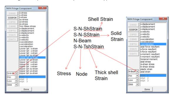
Fig.3: Explanation of the Stress/Strain and node selection for fringing in Frequency Domain Analysis
