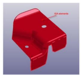
Fig.8: Convert trimmed geometry into trimmed ELMENT\_NURBS\_PATCH elements
