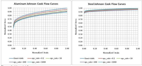
Figure 2. Material flow curves.
