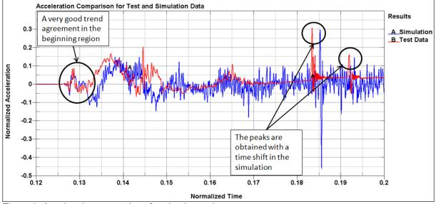
Figure 8. Acceleration comparison for aluminum plate
