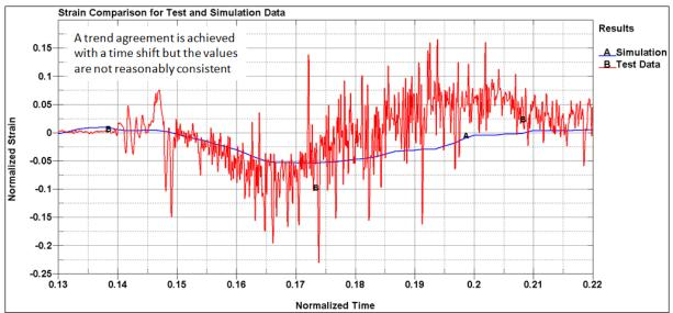
Figure 9. Strain comparison for aluminum plate.
