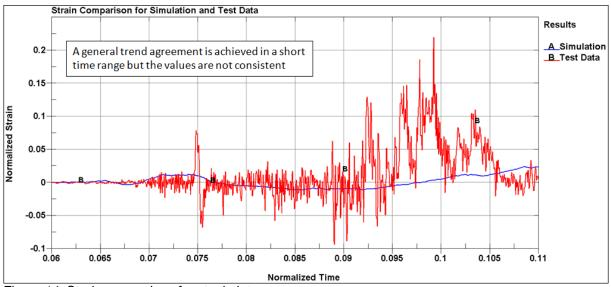
Figure 14. Strain comparison for steel plate.
