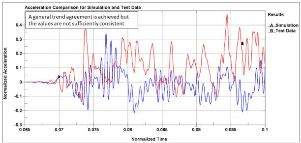
Figure 13. Z acceleration comparison for steel plate.
