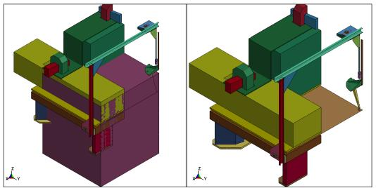
Figure 4. Finite element model of the test plates and setup.
