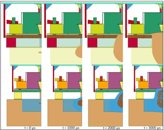
Figure 15. ALE and SPH comparison.
