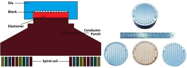
Figure 11: principle (left) and example of flat engraving (right) of indirect MPF.
