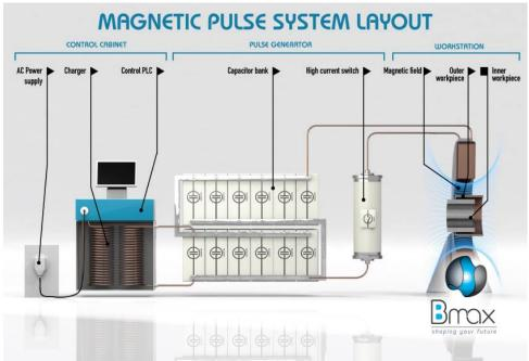
Figure 1 : Process Principle Diagram
