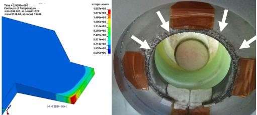
Figure 8: The left picture shows the fringes of temperature obtained in the coil section (steel 40CMD8, melting température is 1671°K, expected welding in red). The right picture presents the real melting zone after 15 shots.
