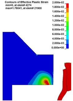
Figure 9: previous coil design with the damage zone.
