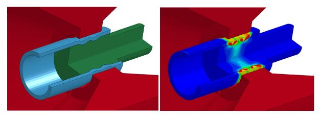
Figure 4 : (left) MPC 3D model, deformed shape (right) equivalent plastic strains in the tube and the anvil at the end of the process.
