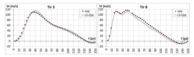
Figure 13: Comparison of radial velocities for an 1050 aluminum tube. The same set of parameters is used for 2 energy levels.
