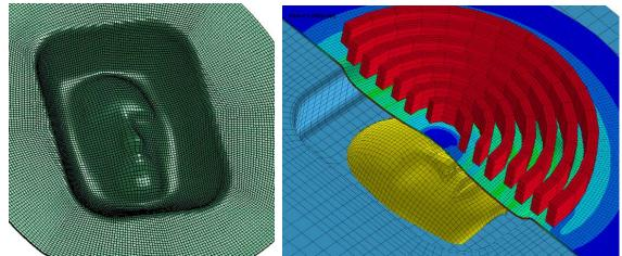
Figure 10: Example of deep drawing with a spiral coil, final shape (left) and Lorentz forces in the workpiece (right)
