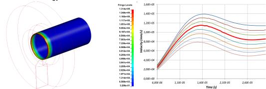
Figure 3: On the left picture, the finite element model with the coil (red part) and the tube with the resultant velocities at 18.5 µs. On the right one, the calculated radial velocity at each millimeter from the tube edge. At 3 mm, the maximum reaches 115 m/s (red curve).
