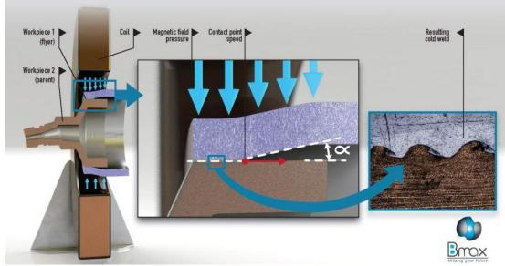
Figure 6: physical principle of MPW
