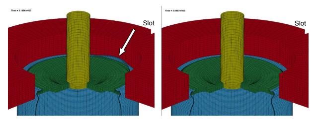
Figure 5 :  $\frac{3}{4}$  cutting view of the crimping set-up with the coil (red), the workpiece (tube in blue), the anvil (green) at 32 µs (left) and 59 µs (right). The white arrow shows the effect of a magnetic field deficiency due to the slot.
