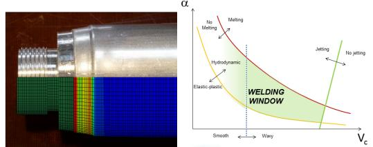
Figure 7: effective plastic strains obtained in the welding zone (left) and the MPW window (right)
