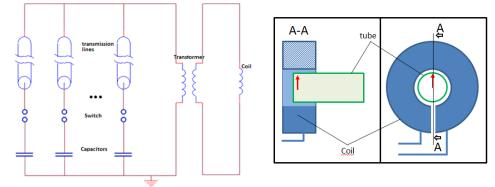
Figure 2 : General electrical circuit (left) and the functional part of the system with the coil (blue), the tube (green) and the PDV (red arrow).
