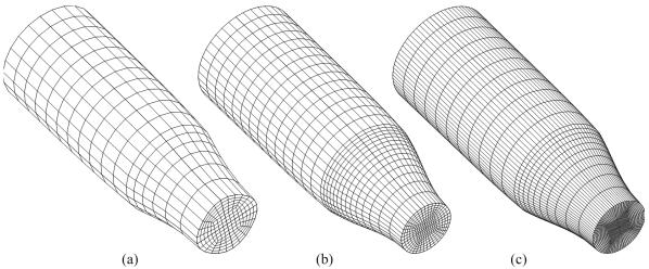
Fig. 3: Three-dimensional cylindrical bar necking. Deformed shapes for the three meshes with 663 (a), 2100 (b) and 6300 (c) elements simulated with the nonlocal regularisation.
