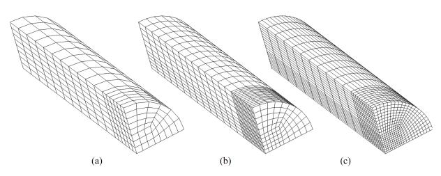
Fig. 1: Three-dimensional cylindrical bar necking. Finite element meshes of 663 (a), 2100 (b) and 6300 (c) elements.
