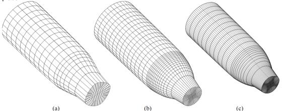
Fig. 2: Three-dimensional cylindrical bar necking. Deformed shapes for the three meshes with 663 (a), 2100 (b) and 6300 (c) elements simulated without the nonlocal regularisation.
