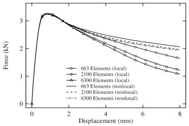
Fig. 4: Force response of the simulations for the 3 different meshes and the two damage models (local and nonlocal).
