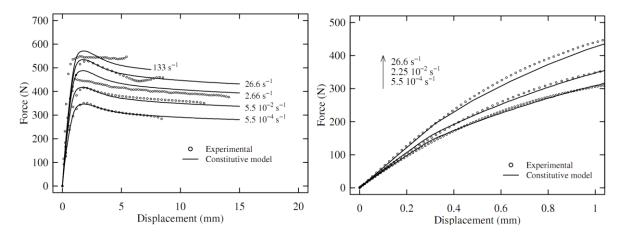
Fig. 6: Experimental vs. constitutive model in uniaxial tensile loading.
