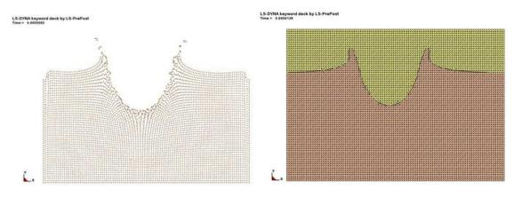
Fig 9. Final deformation shape from SPH model (left) compared to ALE model (right)
