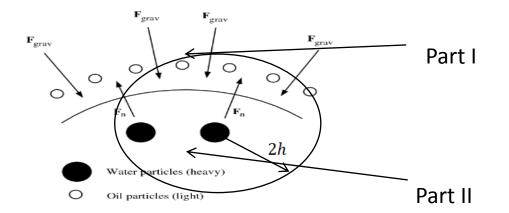
Fig 2. Interaction through SPH interpolation (treated as one part and no contact is needed)
