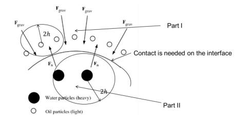
Fig 4. Ineraction through node to node contacts
