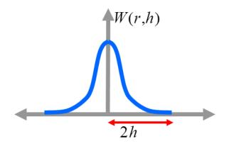
Fig 1. Support size of 2d kennel function
