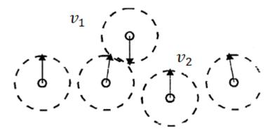
Fig 6. Relative velocity for Linear spring dashpot node to node contacts model
