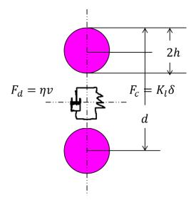
Fig 5. Linear spring dashpot node to node contacts model
