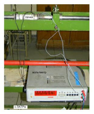
Fig. 1: Heater placed on the rods
