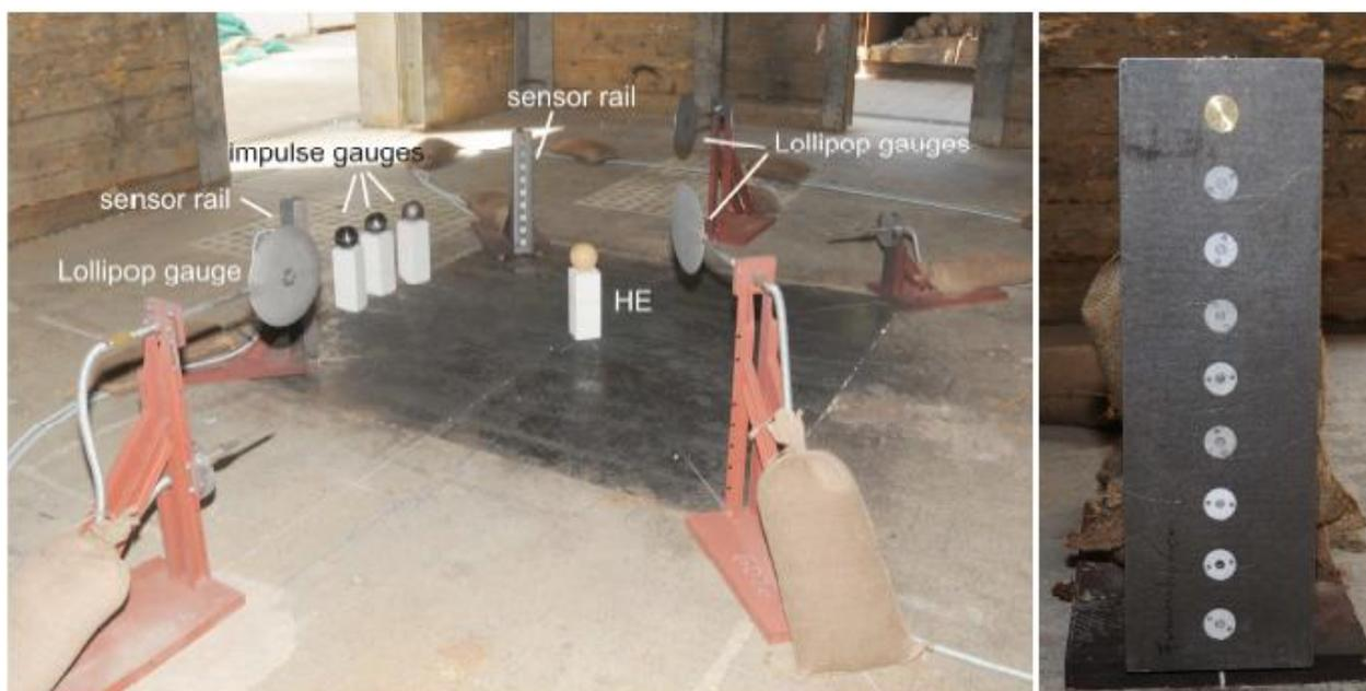
Figure 1 Laboratory test and instrumentation configuration (left) and vertical pressure array right; Figure 3 in Kisters and Kuder (2012).
