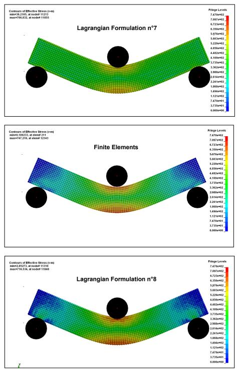
Figure 4 : Von Mises stresses for SPH and Finite Elements models
