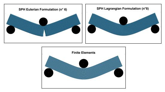
Figure 2 : views of 3-points bending simulations for different types of formulations
