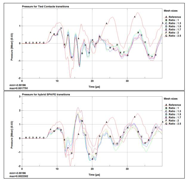
Figure 7 : pressure signals for hybrids and tied contacts transitions
