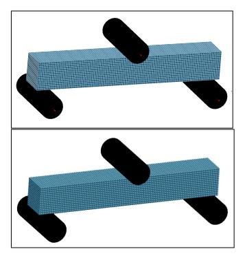
Figure 1 : models of 3-points bending in Finite Elements (at the top) and SPH (at the bottom)
