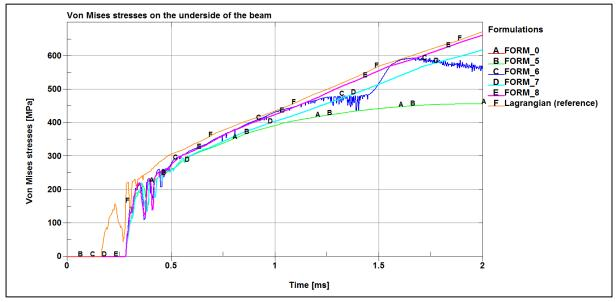
Figure 3 : evolution curves of Von Mises stress under the beam for different formulations
