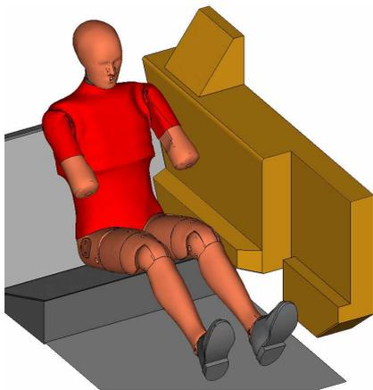
Figure 3. Sled test with D3<sub>P</sub> barrier.
