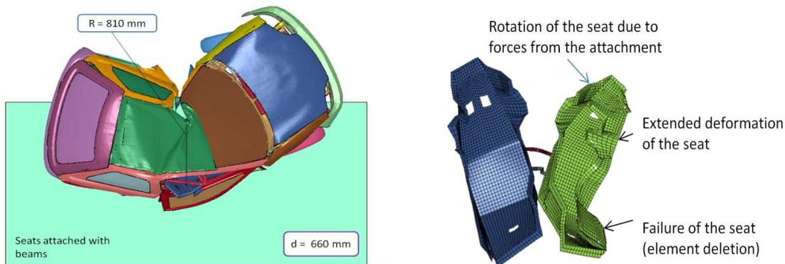
**Figure 12:** deformations of the structure and the seats after the simulation with steel beam attachment
