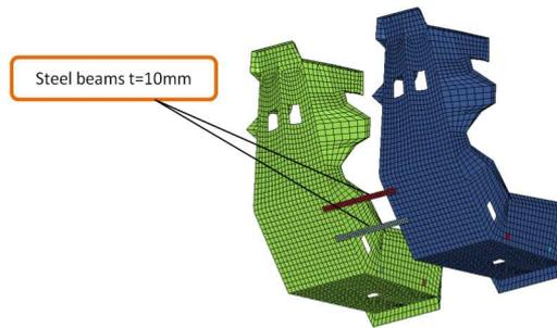
**Figure 10:** Seat attached via two steel beams
