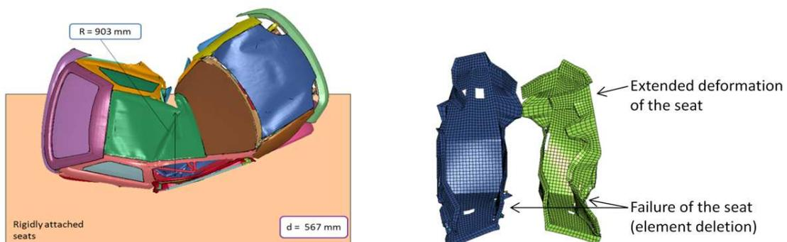
**Figure 11:** Resultant deformations of the structure and the seats after the simulation with rigidly attached rigidly
