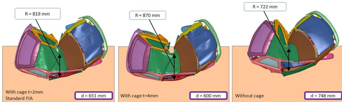
**Figure 6:** Deformation results of the three simulations conducted
