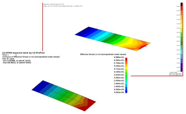
Figure 5 Contour of Von-Mises stress in static analysis by NASTRAN and LS-DYNA
