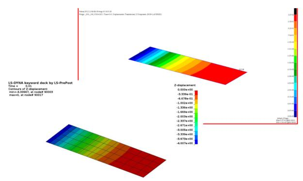
Figure 13 Contour of Z-displacement in direct transient response by NASTRAN and LS-DYNA
