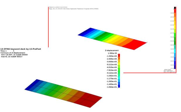
Figure 4 Contour of Z-displacement in static analysis by NASTRAN and LS-DYNA
