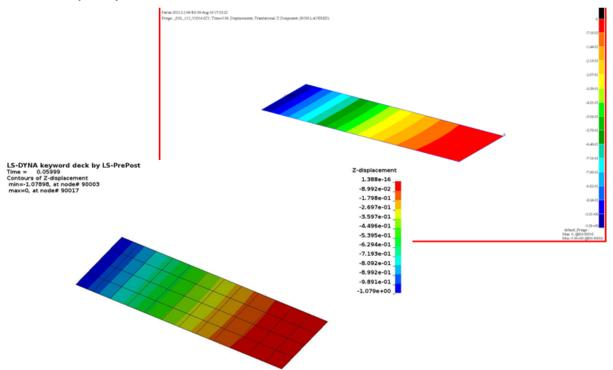
Figure 16 Contour of Z-displacement in modal transient analysis by NASTRAN and LS-DYNA
