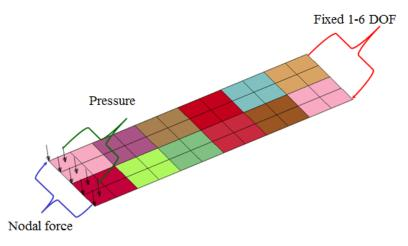
Figure 3 Loads and boundary condition of plate model
