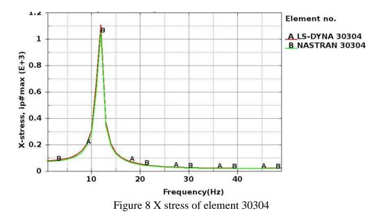
In NASTRAN, modal frequency response analysis is requested by the command SOL 111. The keyword \*FREQUENCY\_DOMAIN\_SSD is used to run the modal frequency response solver in LS-DYNA. Two types of harmonic loads (pressure and nodal force) are applied to the plate simultaneously, one edge of which is fixed (figure 3).
