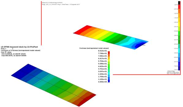
Figure 10 Contour of X stress in modal frequency response by NASTRAN and LS-DYNA
