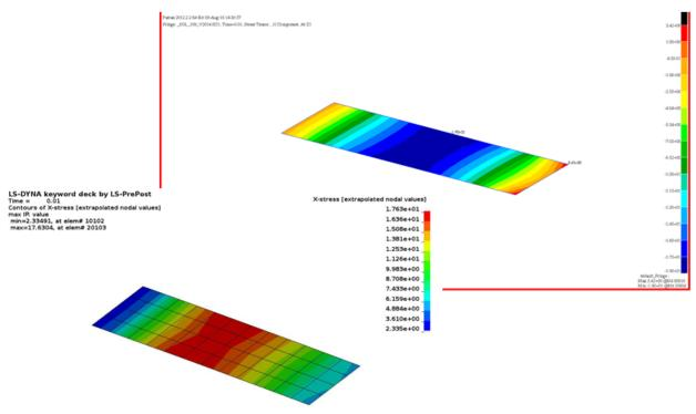
Figure 14 Contour of X stress in direct transient response by NASTRAN and LS-DYNA
