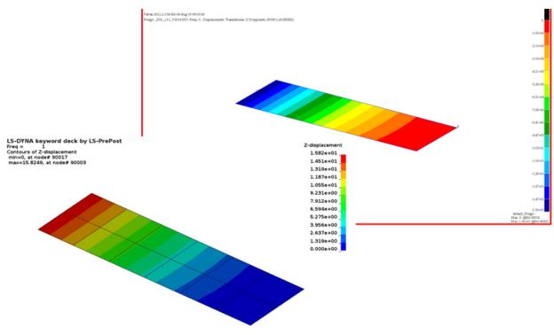
Figure 9 Contour of Z-displacement in modal frequency response by NASTRAN and LS-DYNA
