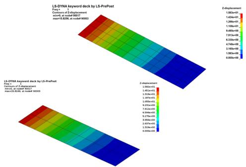
Figure 6 Contour of Z-displacement by mode based SSD and direct SSD in LS-DYNA
