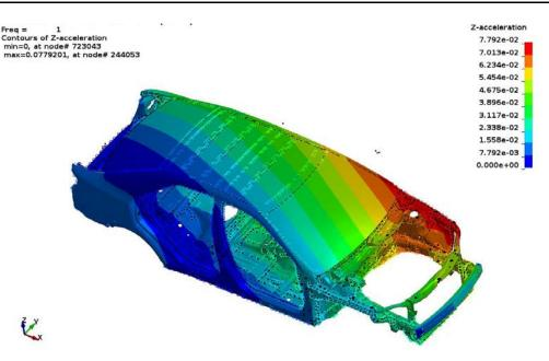
Figure 7. Z acceleration at 1 Hz by MCMS method
