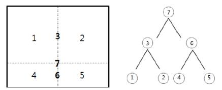
Figure 1. A plate FE model partitioned with two level and the substructure tree topology
