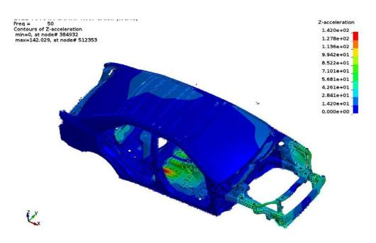
Figure 8. Z acceleration at 50 Hz by Lanczos method
