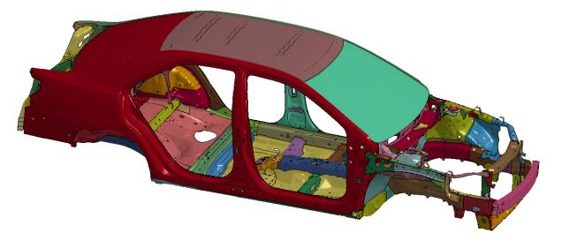
Figure 2. The finite element model of 2012 TOYOTA Camry (NCAC)
