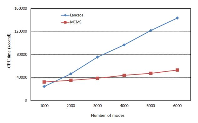
Figure 3. Comparison of CPU time between Lanczos and MCMS
