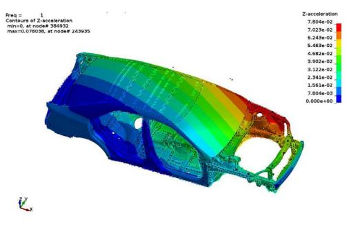
Figure 6. Z acceleration at 1 Hz by Lanczos method
