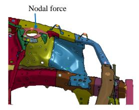
Figure 5. A nodal force applied to the BIW model
