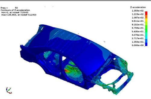
Figure 9. Z acceleration at 50 Hz by MCMS method
