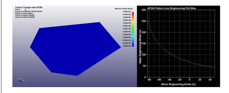
Figure 5a: initial blank shown alongside limit strain diagram for fracture. Strain is engineering and plotting is described below.
