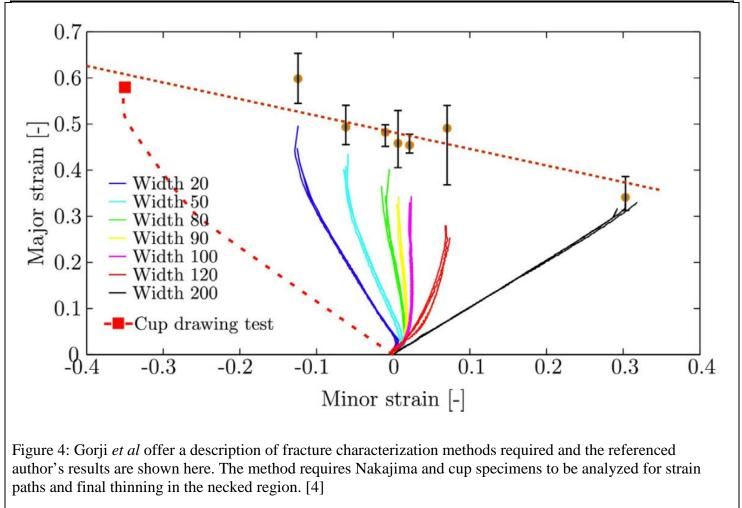
The Linear Fracture Line seen in the above figure 4 is used for fracture definition as was described in the modelling approach section. LS-DYNA demands input of these fracture major strain and minor strain combination in *engineering strain* and thus becomes curvilinear. The resulting simulation using the modelling approach will subsequently be covered in the following section.
