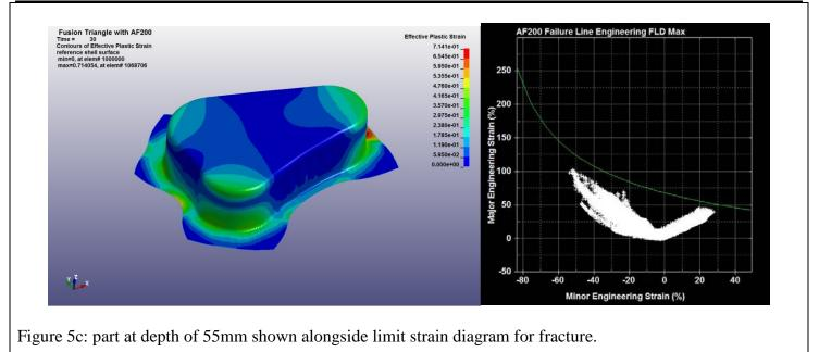
Post processing of the simulation has been performed in LS-PrePost, using its ability to optionally plot engineering strains as opposed to true strains on the FLD. LS-PrePost offers the user the option to specify the same curve as was used in the failure definition as LCFLC.
