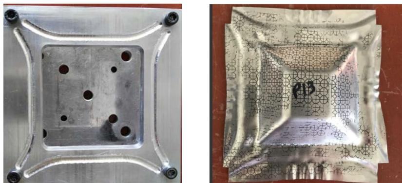
Figure 8. (Left) Binder with drawbead and (right) the resultant component without wrinkles.
