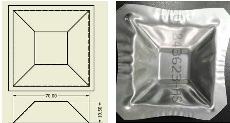
Figure 1. (Left) Drawing, not to scale, of the studied component, and (right) picture of one stamped part without drawbeads.
