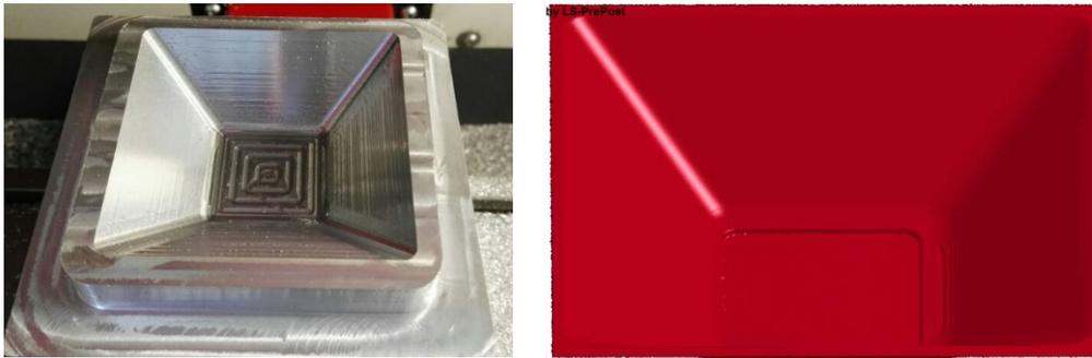
Figure 3. Physical die (left) and its digitized 3D model (right) imported in LSPP.
