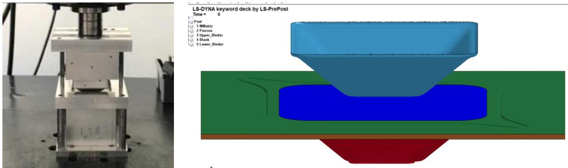
Figure 4. (Left) Stamping dies mounted in the Universal Testing Maching, (right) Stamping model at initial position.
