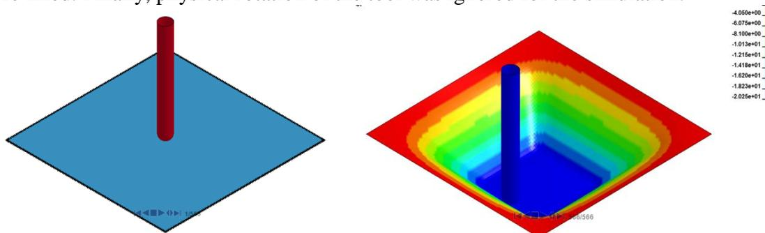
Figure 2. (Left) Initial ISF model, and (right) final deformation state.
