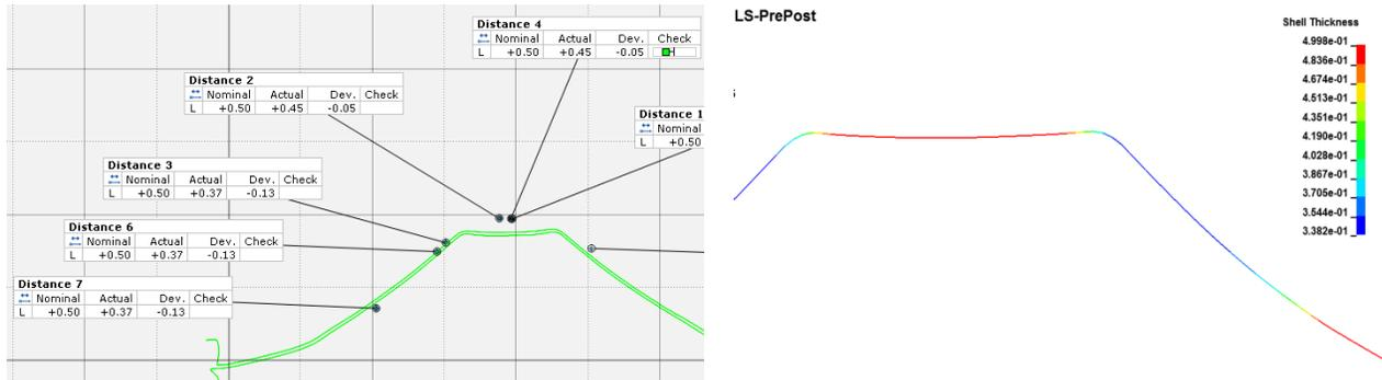
Figure 6. (Left) Thickness measurements on one fabricated part. (Right) Model shell thickness.
