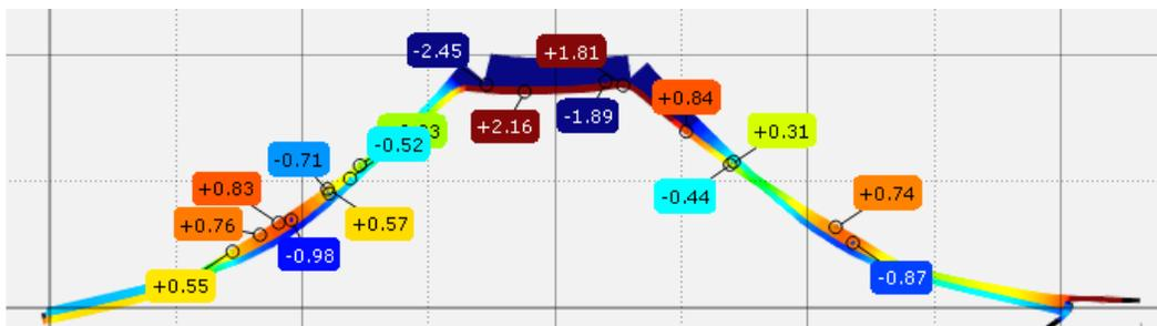
Figure 5. Geometric deviation, in mm, between the physical and virtual parts.
