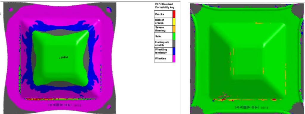
Figure 7. Formability of the Stamped component without (left) and with (right) drawbeads.
