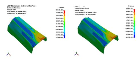
Figure 2: The one-step solutions using finite elements (left) and trimmed NURBS (right).
